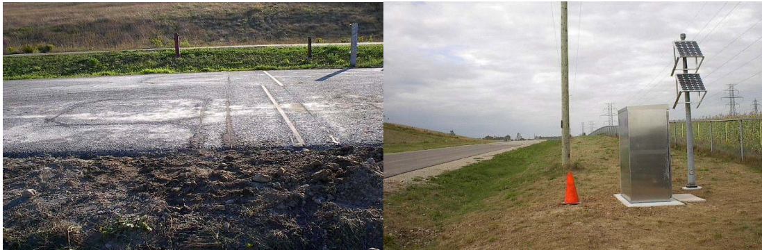
Figure 3.4: CPATT Piezoelectric Sensors and Roadside Cabinet
