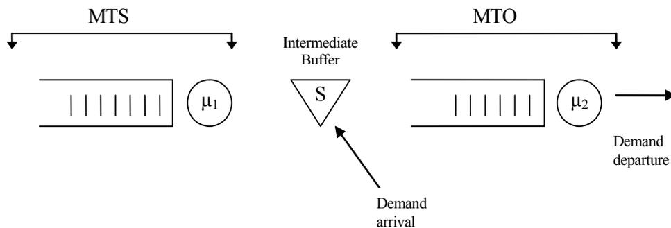
Figure 1.1: A Typical Hybrid Manufacturing System
