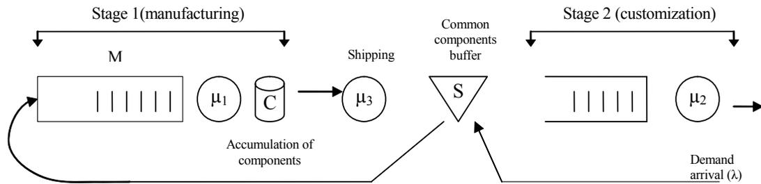
Figure 4.1: Hybrid MTS-MTO system with batch replenishment policy
