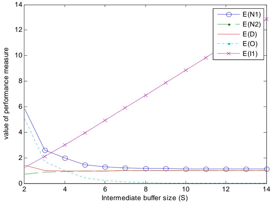
Figure 3.3: Performance evaluation with various buffer sizes
