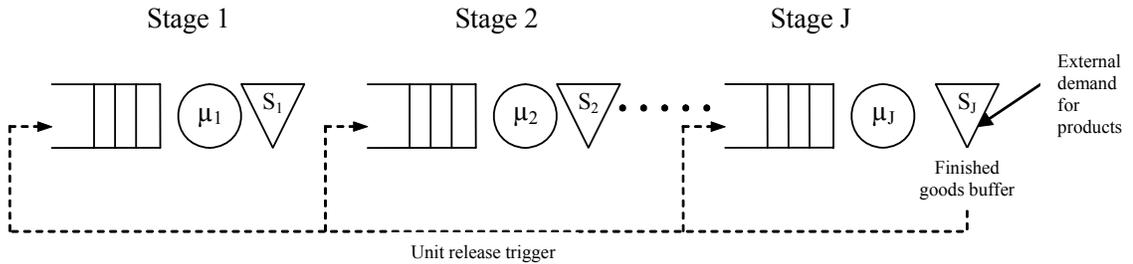
Figure 2.1: A schematic representation of a multi-stage P/I system
