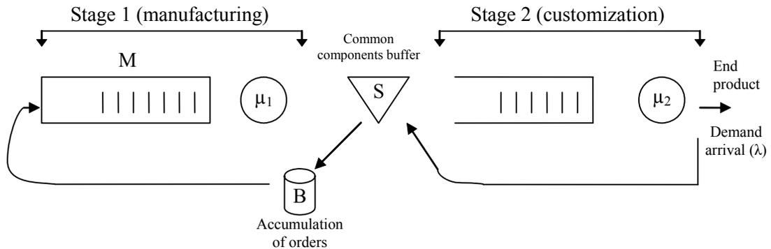
Figure 3.1: The MTS-MTO system with batch ordering policy
