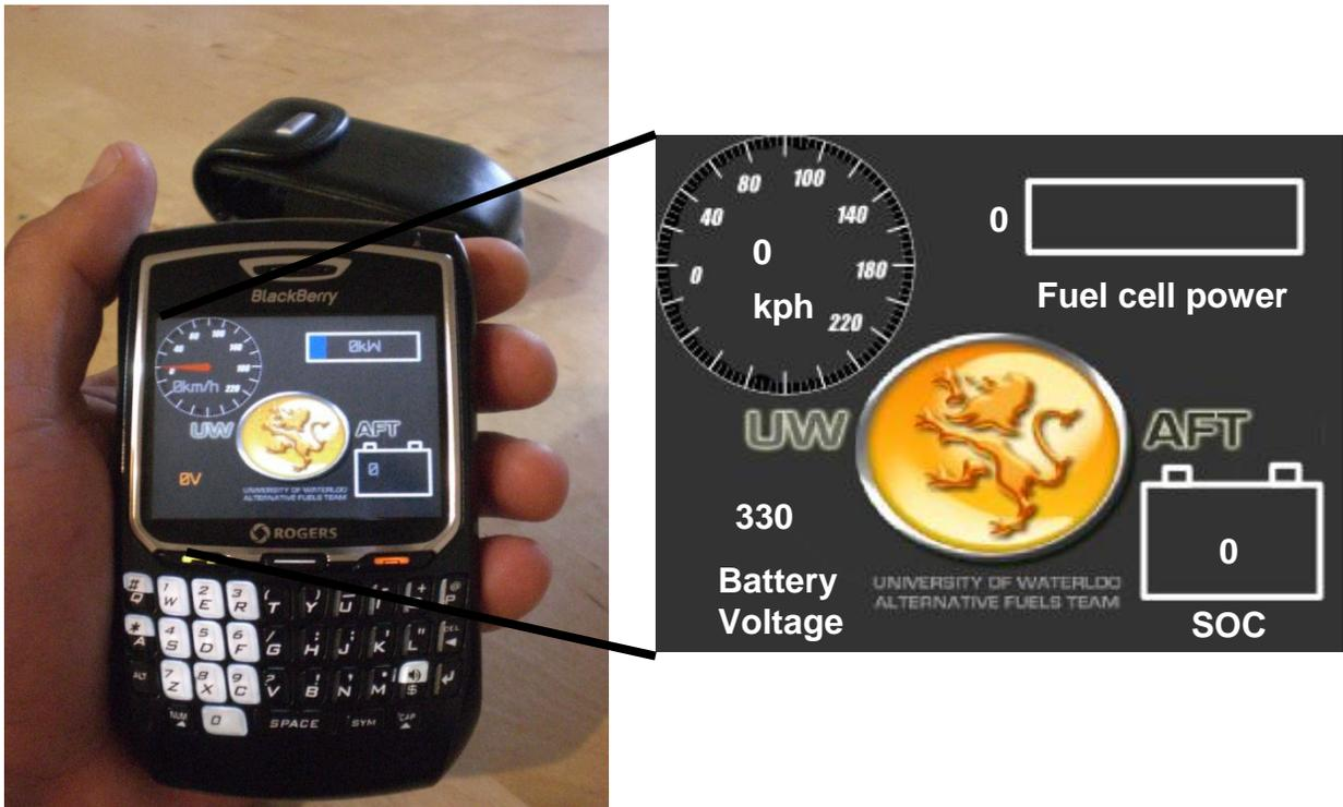
Figure 64: Bluetooth CAN message receiver on the Blackberry™ device
