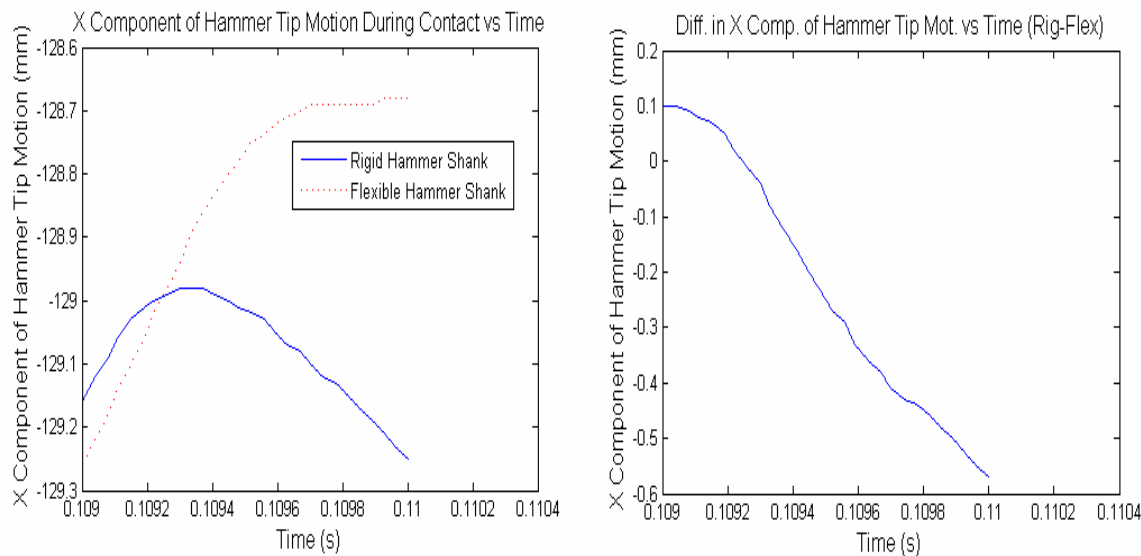
Figure 4.7: X Component of the Displacement of the Hammer Head Tip
