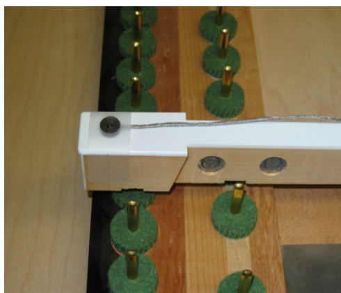
Figure 2.3: Load Cell Mounted on the Key
