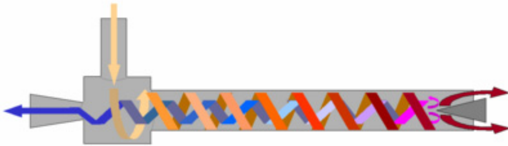
Figure 3.7. Design of a Vortex cooler. Pressurized air (vertical arrow) enters the tube at a right angle. Air molecules with high kinetic energy exit the back of the tube as hot air (maroon arrows); air molecules with lower energy (blue) travel through the centre of the tube and are ejected through the nozzle as a stream of cool air [10].
