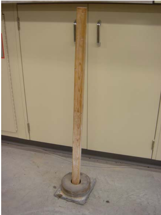
Figure 6.15: The hand-held hammer (15 lbs) used to compact slab 2
