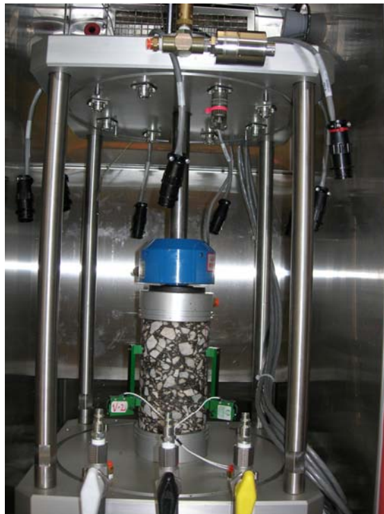
Figure 5.18: Dynamic modulus test setup
