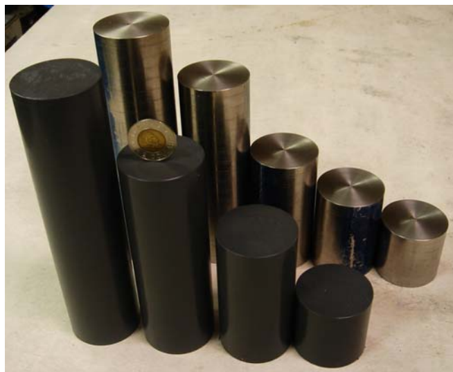
Figure 5.10: PVC and steel standard test blocks for calibration
