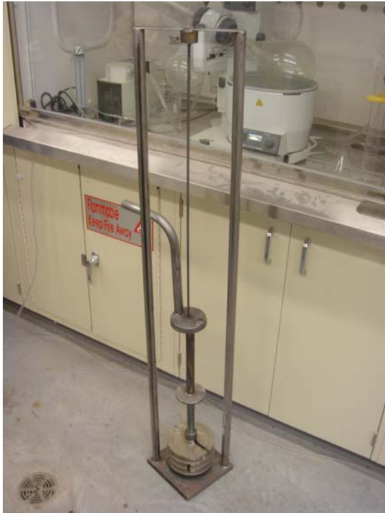
Figure 6.32: The modified compactor (35 lbs) used in slab 3 fabrication
