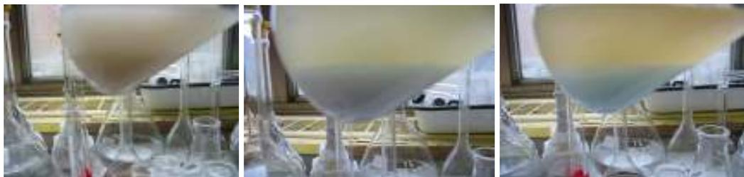
Take 10ml above LAS/LAB solution, add 20ml H<sub>2</sub>O, 15ml chloroform , 1ml 0.01N H<sub>2</sub>SO<sub>4</sub> and 5ml **DY**.
