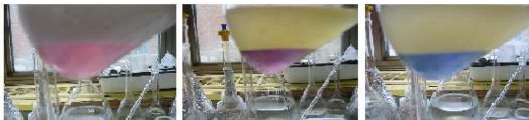
Figure 4.1: The color changes of the titration of low LAS concentration solution, using mixed indicator as indicator.
