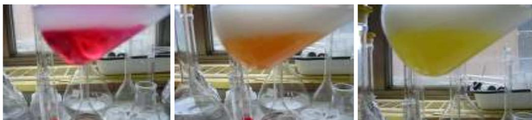
Figure 4.4: The color changes of the titration of low LAS concentration solution, using dimethyl yellow as indicator
