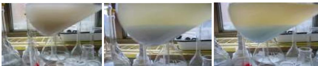
Figure 4.3: The color changes of the titration of low LAS concentration solution, using mixed indicator as indicator.
