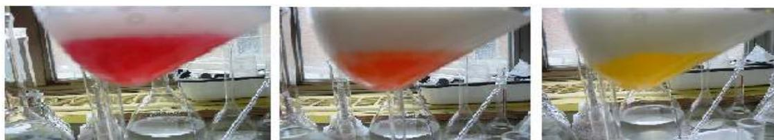
Figure 4.2: The color changes of the titration of high LAS concentration solution, using dimethyl yellow as indicator.
