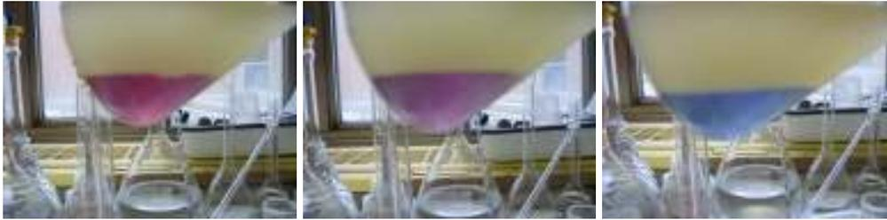
Take 0.3ml LAS/LAB solution, add 20ml H<sub>2</sub>O, 15ml chloroform , 1ml 0.01N H<sub>2</sub>SO<sub>4</sub> and 5ml **DY**.
