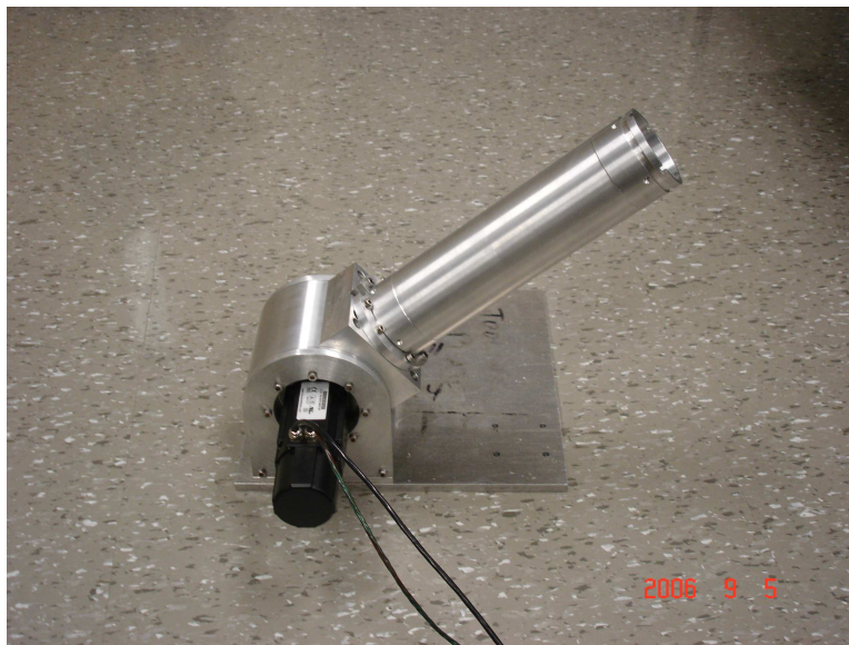
Figure 2.5: MRR rotary joint built at UW
