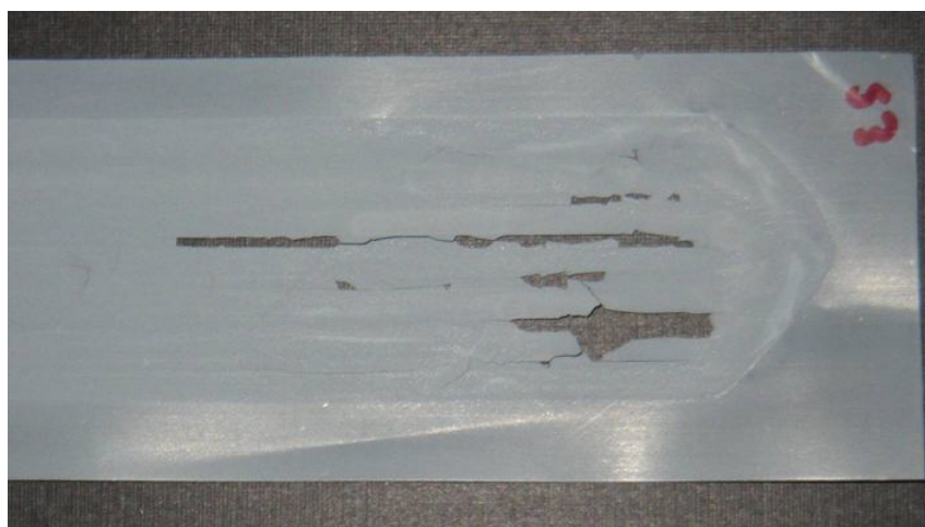
Figure 6-28: Cracking of membrane 16 after 300 hours of operation on HTDS.
