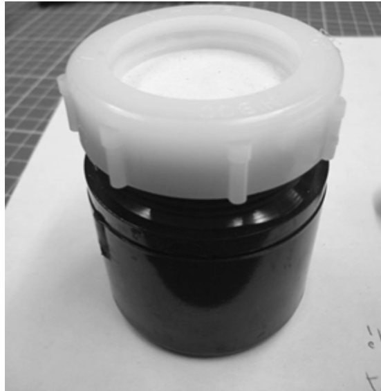
Figure 2-2: Cup test equipment for static water permeation test.
