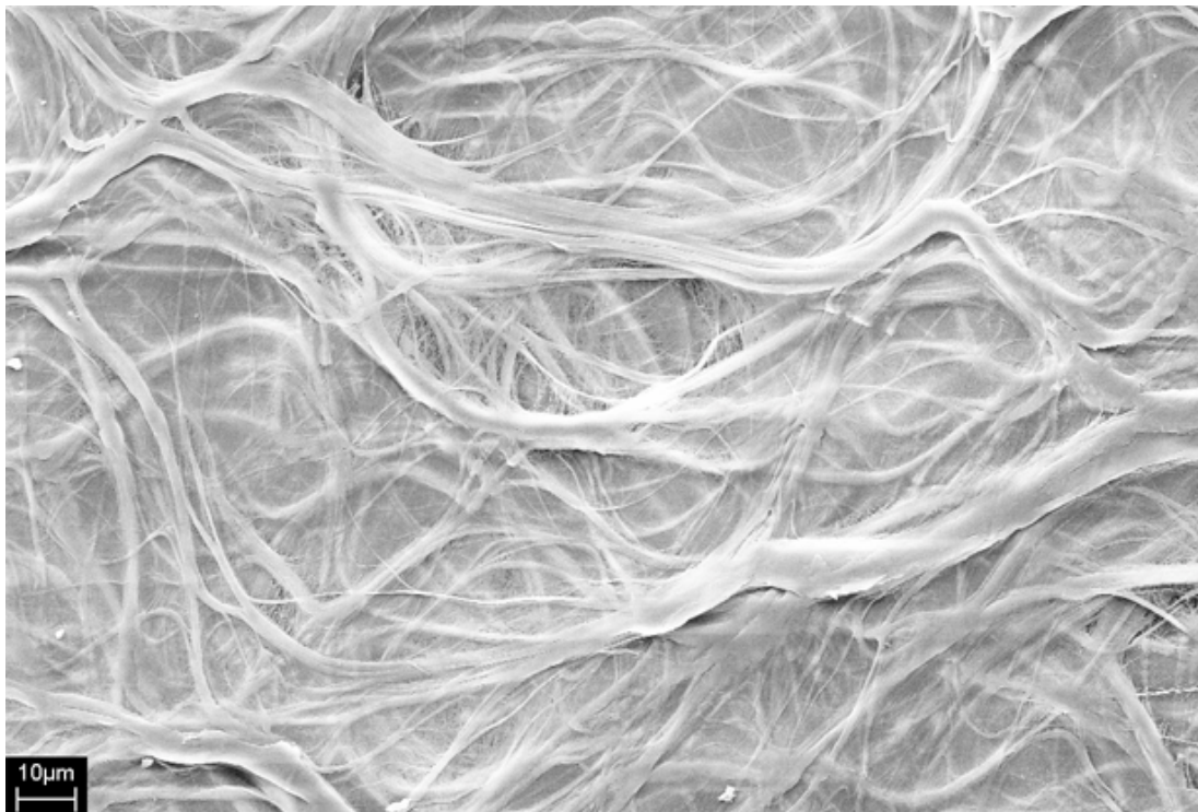
Figure 6-11: Membrane 12 at 1000x magnification after 1146 hours of operation on HTDS under SEM.
