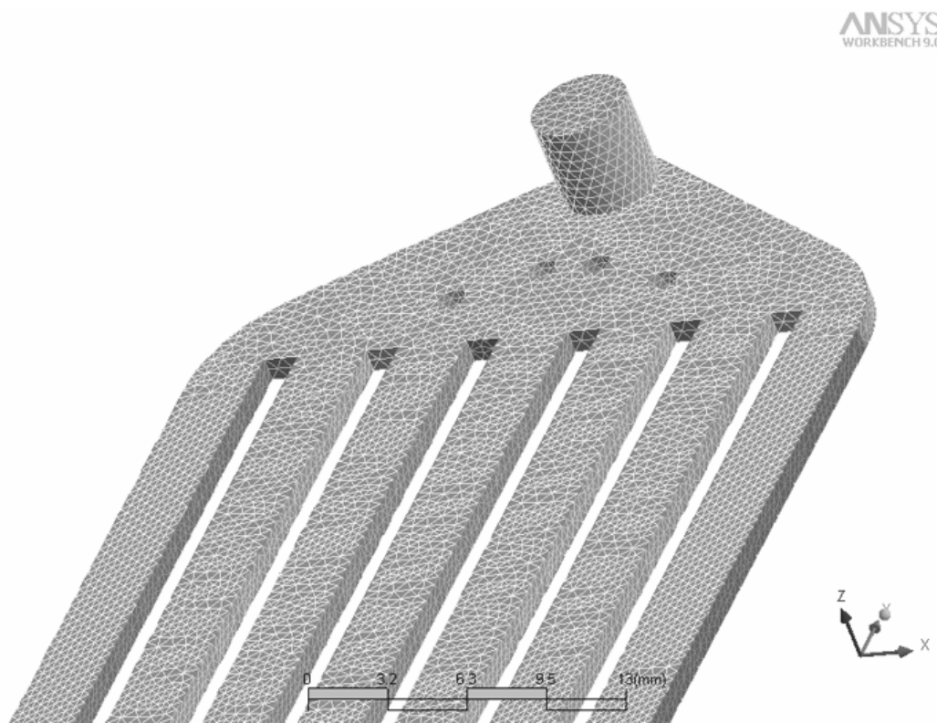
Figure 2-6: Surface mesh of solid model of flow channels for the water permeation test module in ANSYS Workbench™ 9.0.
