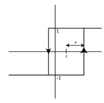
Figure 2.9: A Relay of Centre s and Half-Width r
