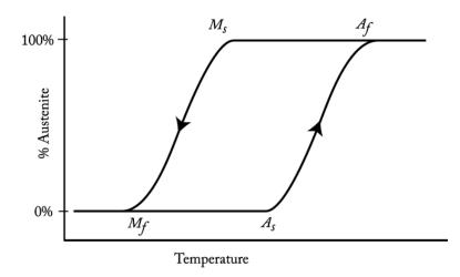
Figure 2.1: SMA Phase Transition Hysteresis Loop
