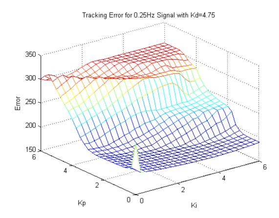
Figure 6.4: Tracking Error for 0.25Hz Reference Signal with  $K_d{=}4.75$
