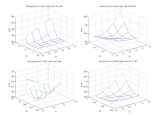
Figure 6.2: Cost Functions Near Optimal Controllers
