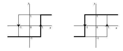
Figure 2.5: Relay Output
