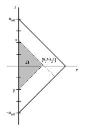
Figure 2.14: Region  $\Omega$  Corresponding to Output Change  $y_{\alpha} - y_{\alpha\beta}$
