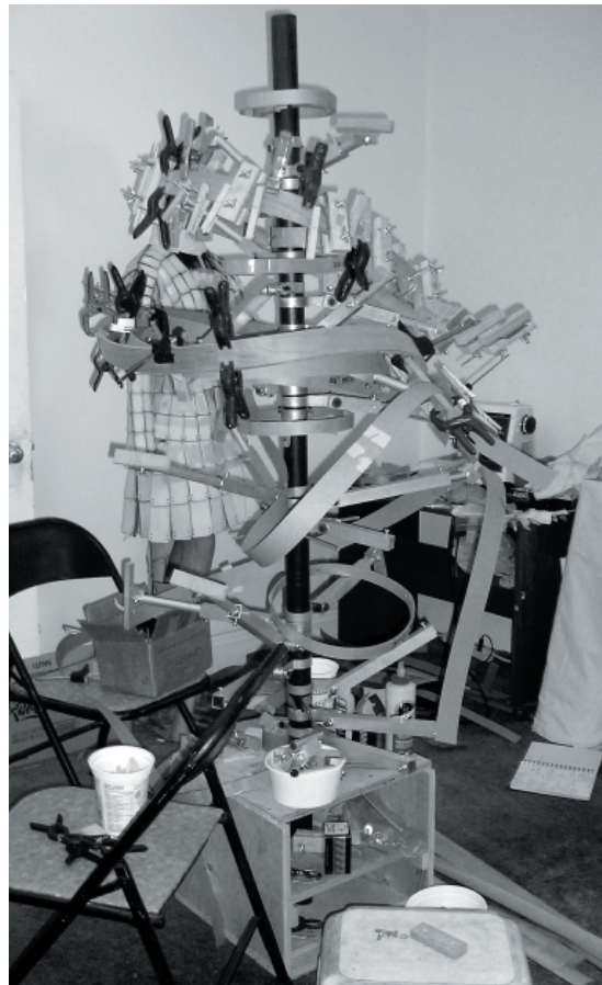
100 Wood Dress (in progress), June 2006. 1/16" Black cherry veneer. Drying, gluing, and clamping ribs during the lamination process. Each rib is 3 ply for a total thickness of 3/16".
