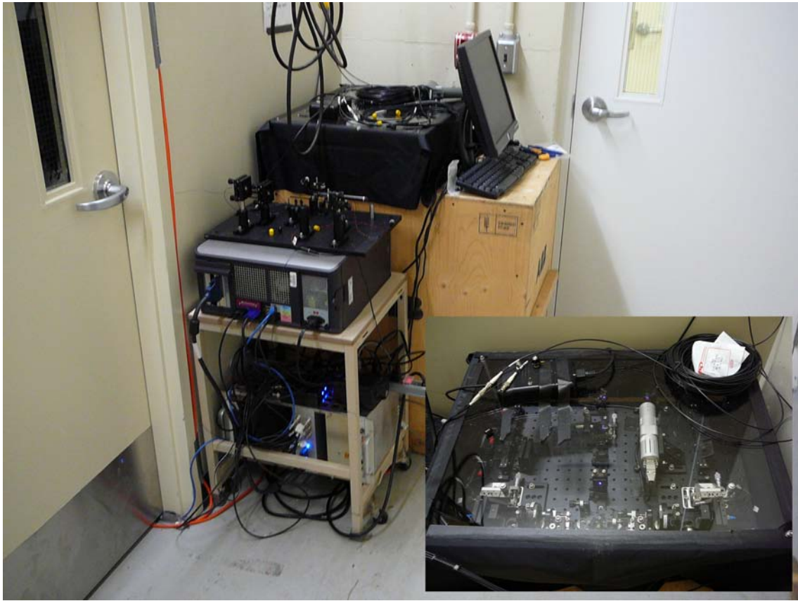
Figure 2.4: Portable entangled photon source sitting on the 6th floor of the CEIT building.
