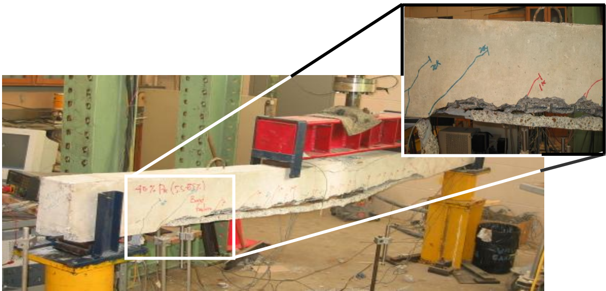
Figure 6.4: Fatigue bond failure of the 40% prestressed strengthened beam
