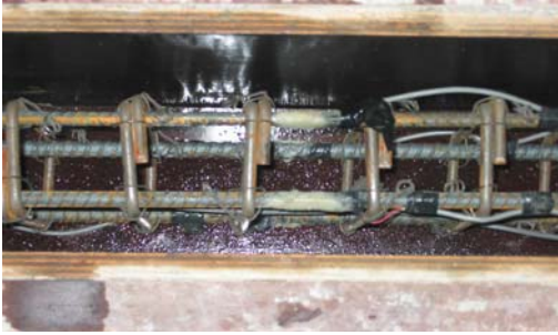
Strain gauges mounted on steel
