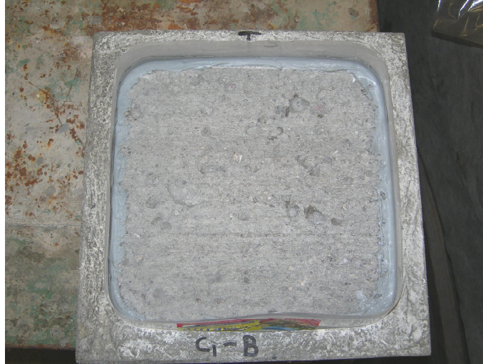
Figure 4-36, C 1 concrete slab used for salt scaling test after 55 freeze-thaw cycles.
