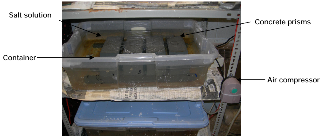
Figure 3-10, The container and prisms for corrosion experiments.
