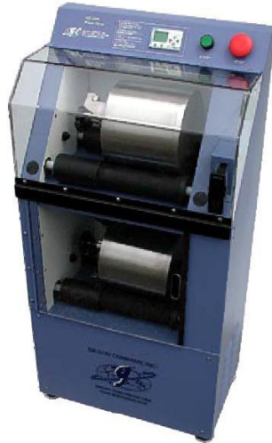
Figure 3-7, Micro-Deval instrument used for aggregate abrasion resistance test [27].
