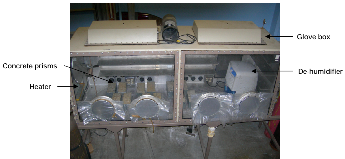
Figure 3-11, A perspective of the chamber used for drying the concrete prisms.
