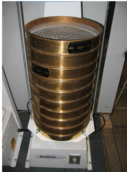
Figure 3-5, Superimposed sieves used for grading the aggregates.
