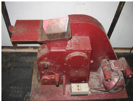
Figure 3-4, The laboratory crushing machine used for producing the OC-RCA.
