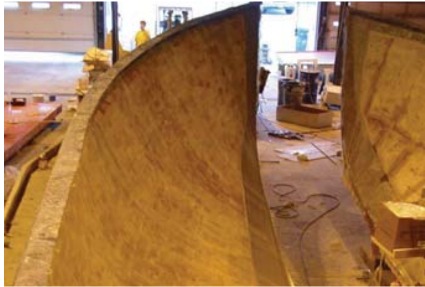
56. Directional layers of fiberglass laminated to a formed balsa core
