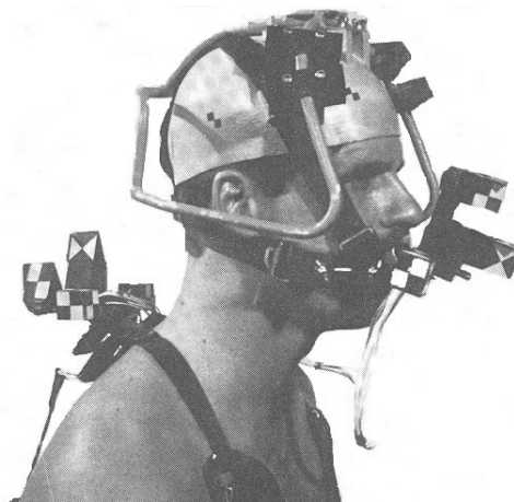
Figure 8-2: Instrumented Human Volunteer for the NBDL Sled Test Experiments
