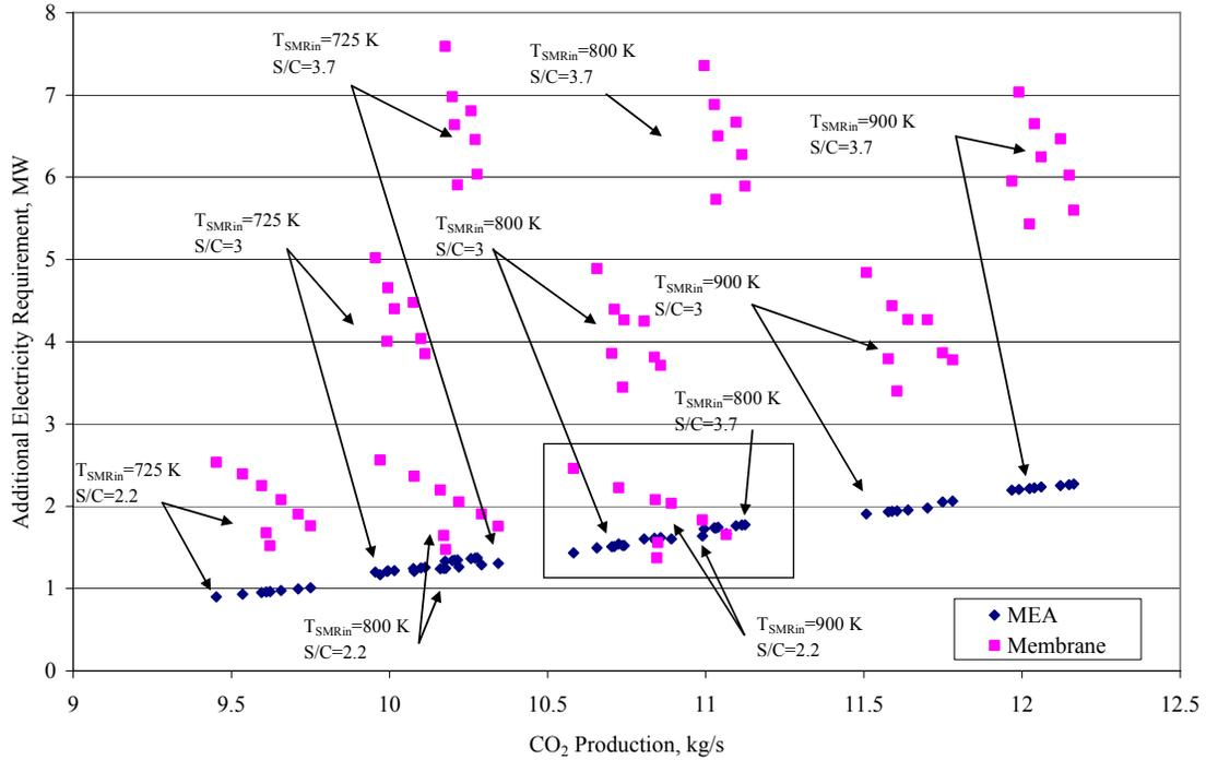
**Figure 4.5: Sensitivity of additional electricity requirement of CO<sub>2</sub> capture process to CO<sub>2</sub> production**
