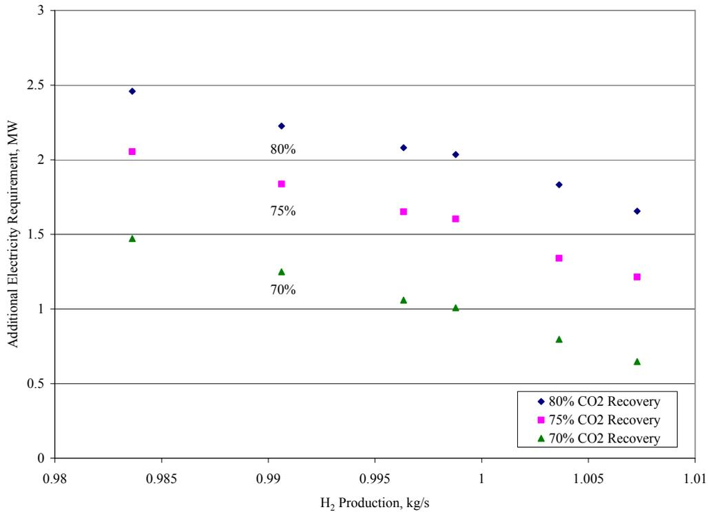
**Figure 4.7: Sensitivity of additional electricity requirement to percent CO<sub>2</sub> recovery (Membrane)**
