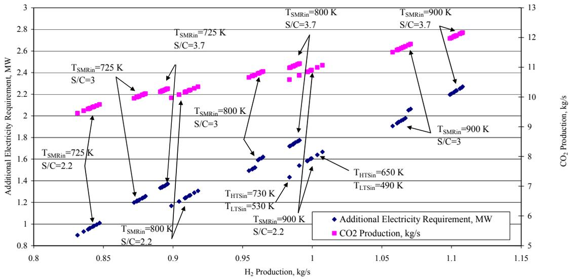
**Figure 4.2: Sensitivity of additional electricity requirement and CO<sub>2</sub> production to H<sub>2</sub> production (MEA)**
