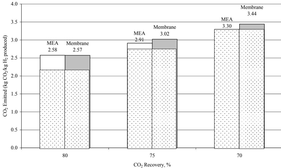
**Figure 4.8: Comparison of CO<sub>2</sub> emissions to the atmosphere at various CO<sub>2</sub> recoveries**
