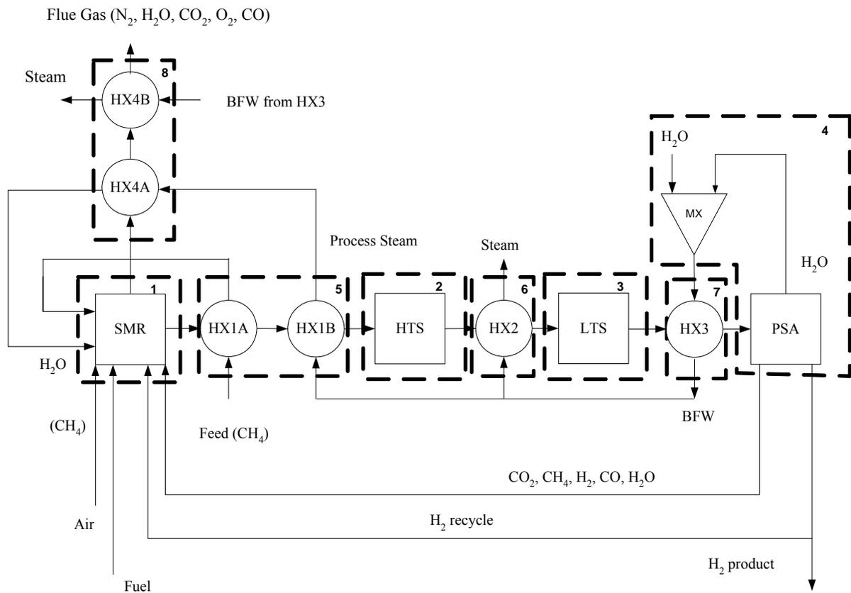
**Figure 3.1: H<sub>2</sub> plant without CO<sub>2</sub> capture**
