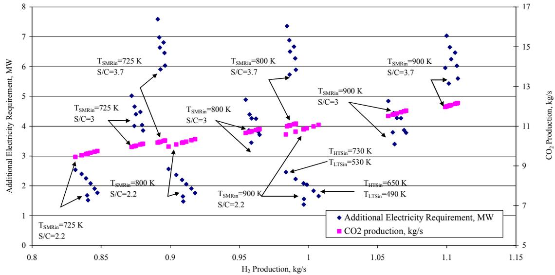
**Figure 4.3: Sensitivity of additional electricity requirement and CO<sub>2</sub> production to H<sub>2</sub> production (Membrane)**
