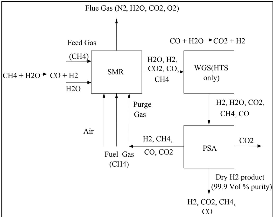
**Figure 2.3: Typical H<sub>2</sub> plant – PSA (1970s – mid 1980s)**
