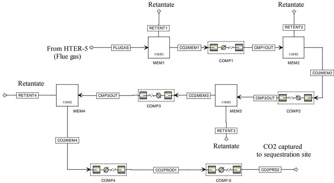
**Figure 3.16: H<sub>2</sub> plant with membrane separation technology**
