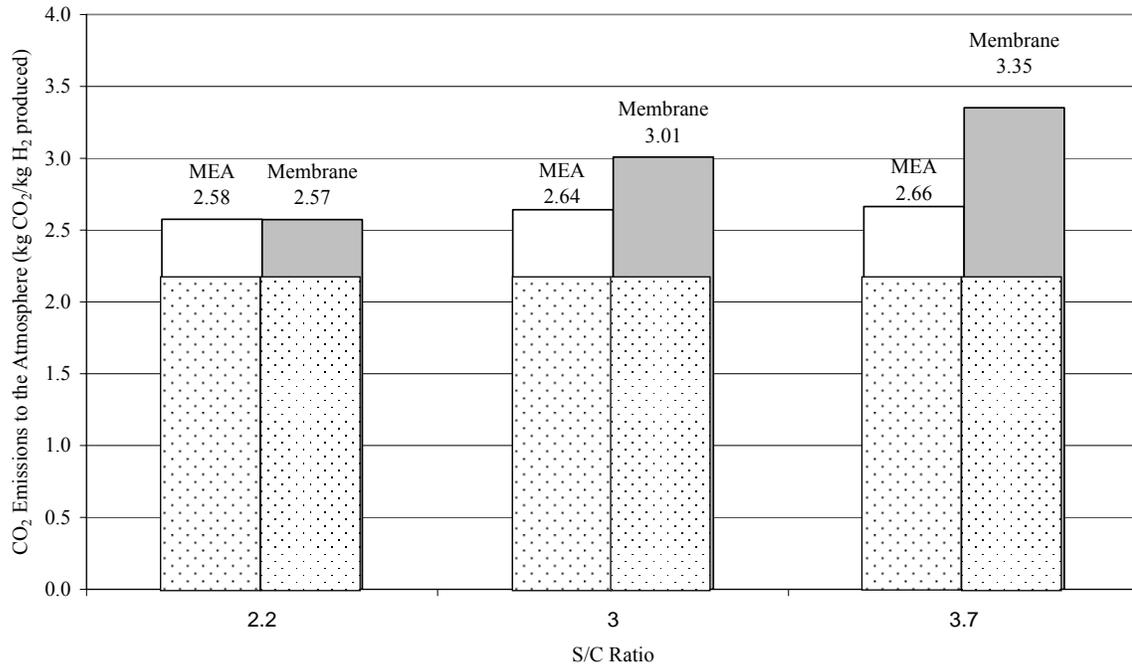
**Figure 4.4: Comparison of CO<sub>2</sub> emissions to the atmosphere:  $T_{SMRin} = 900$  K,  $T_{HTSin} = 570$  K  $T_{LTsin} = 490$  K**
