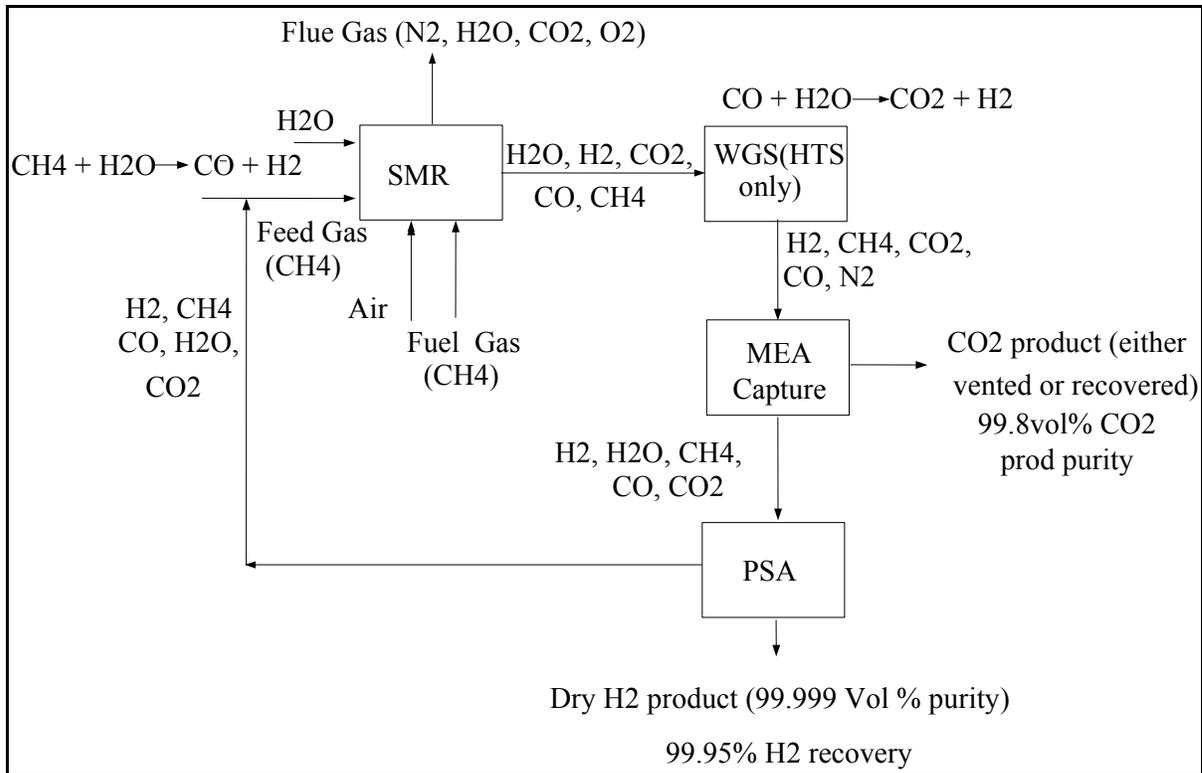
**Figure 2.4: Latest H<sub>2</sub> plant – MEA + PSA (1980s - present)**
