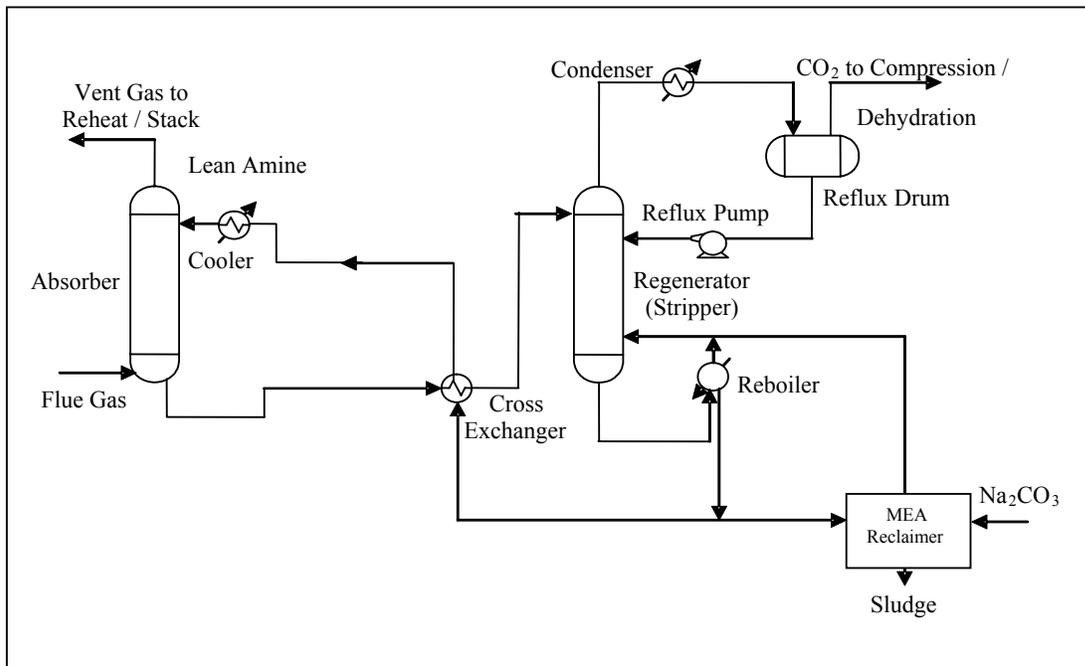
**Figure 2.5: Basic process flow diagram for MEA-CO<sub>2</sub> capture process**
