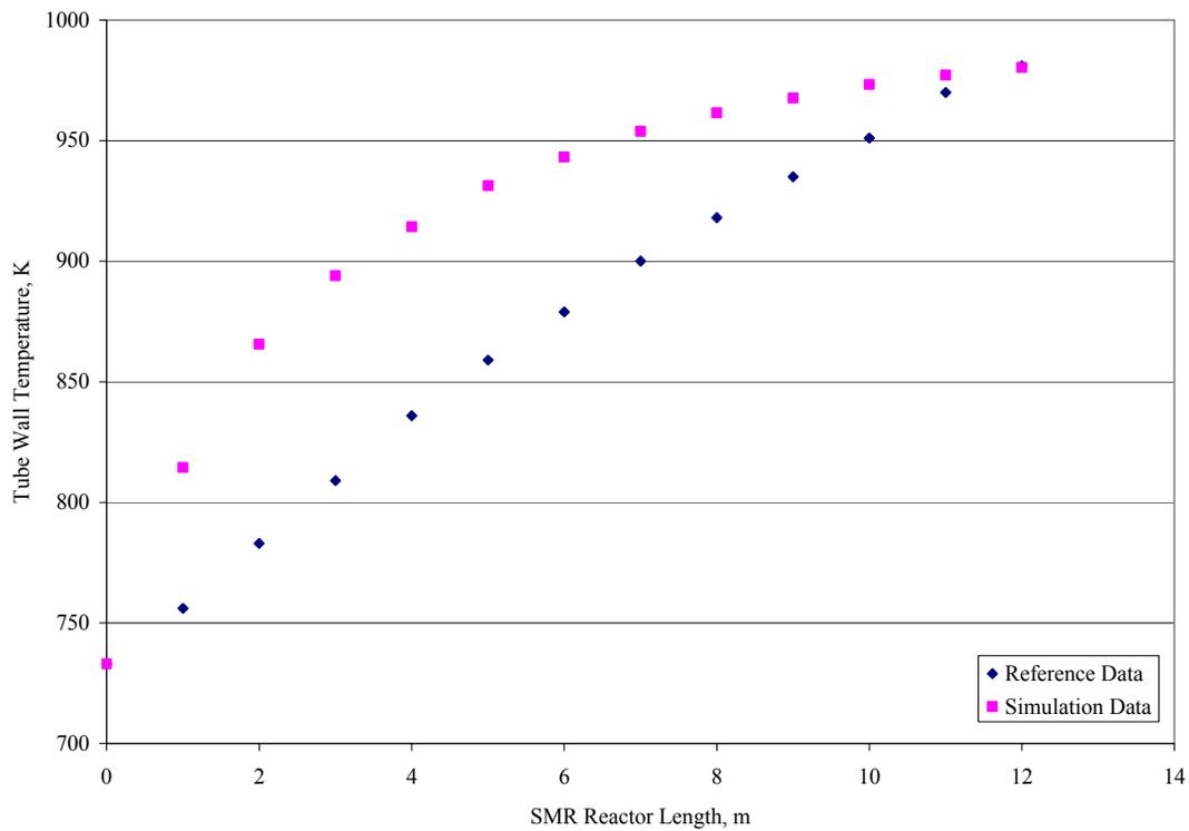
**Figure 3.3: Tube wall temperature profile of SMR**
