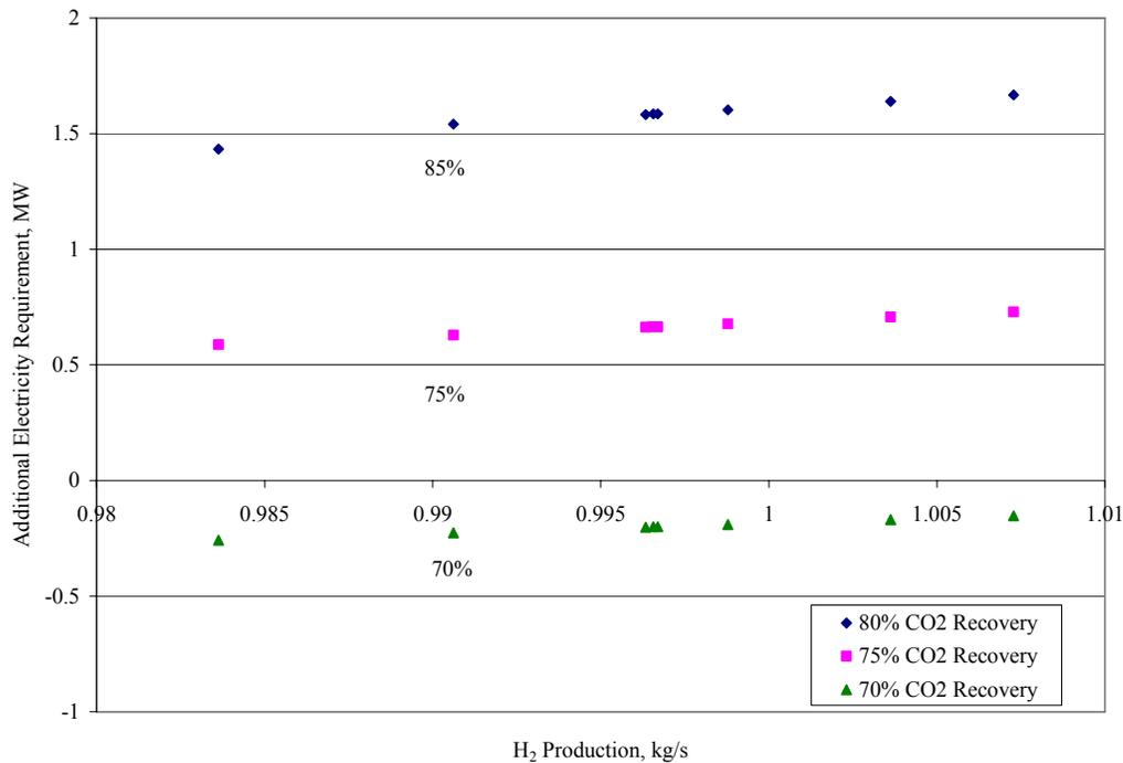
**Figure 4.6: Sensitivity of additional electricity requirement to percent CO<sub>2</sub> recovery (MEA)**
