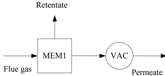
**Figure 3.15: One-stage membrane separation process**
