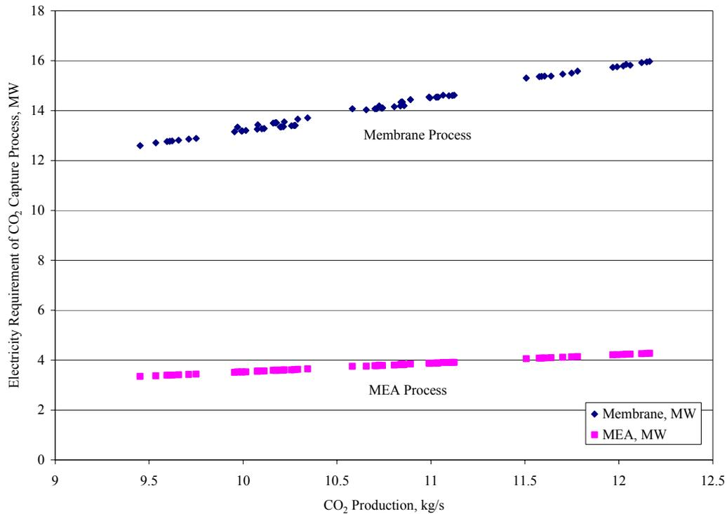
**Figure 4.1: Sensitivity of electricity requirement of CO<sub>2</sub> capture process to CO<sub>2</sub> production (case of 80% CO<sub>2</sub> capture from the furnace of the SMR)**
