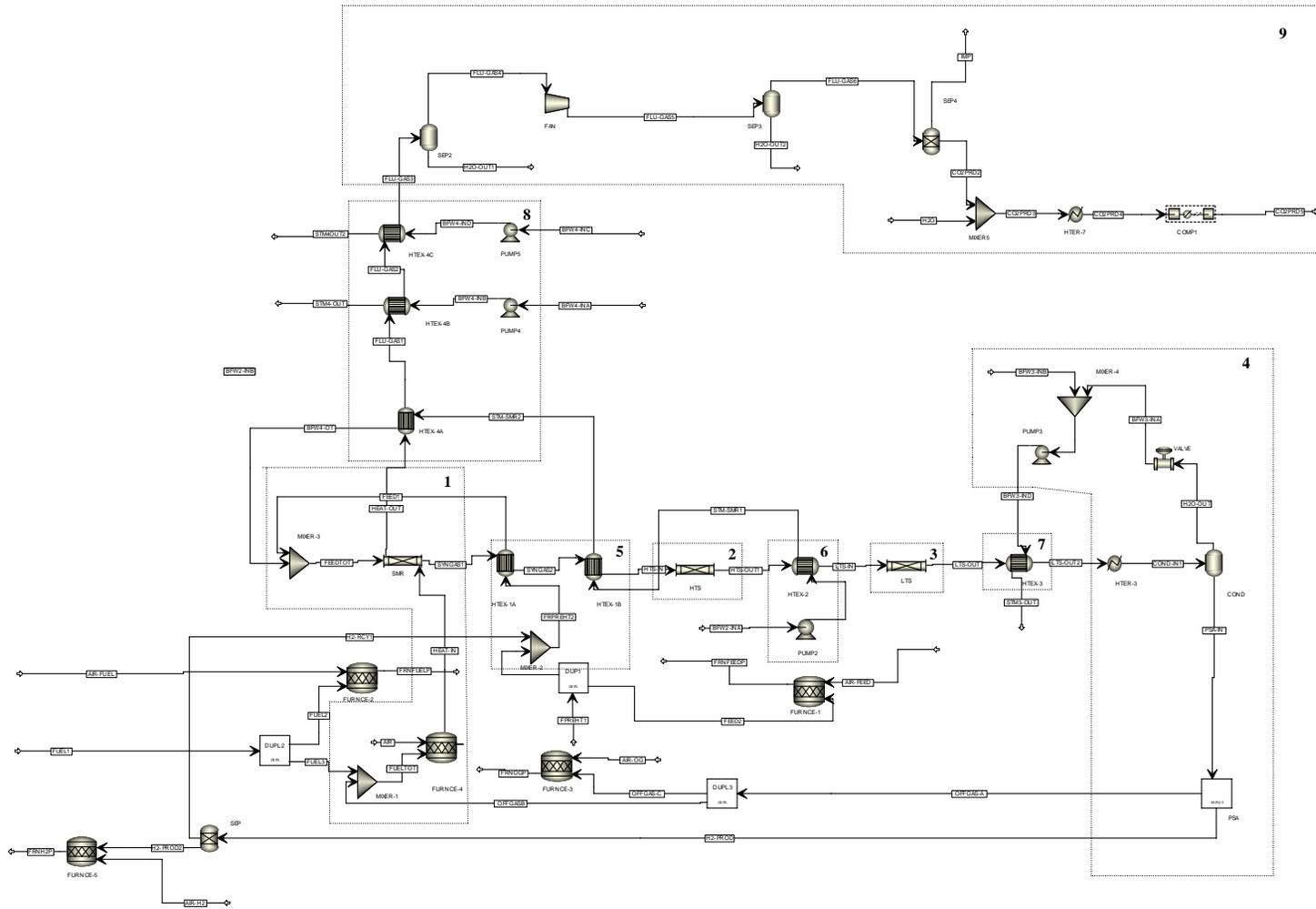
Figure 3.13: H<sub>2</sub> Plant with simulation in approximating the amount of electricity needed by the MEA capture plant
