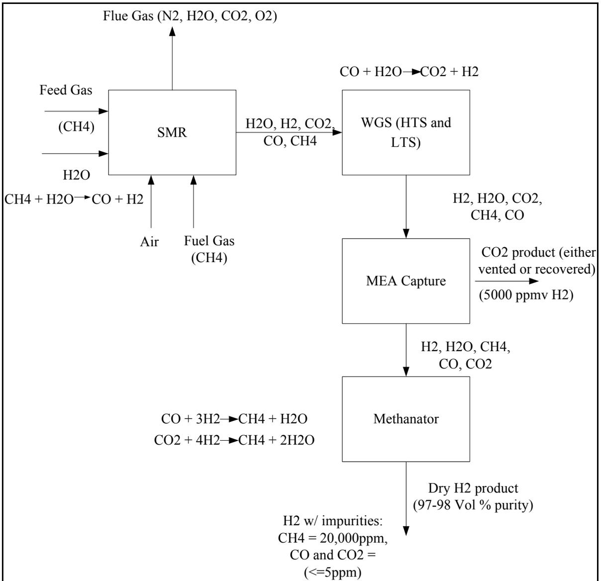
**Figure 2.2: Conventional H<sub>2</sub> plant - MEA (1960s – mid 1970s)**
