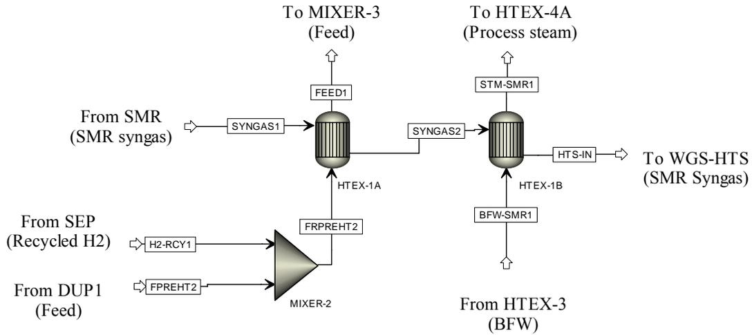
**Figure 3.8: Block #5 - SMR syngas heat exchange system**
