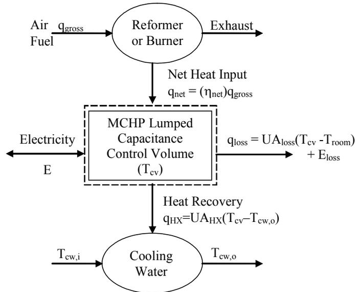
**Figure 4-1 Generalized MCHP Model Energy Flowchart**
