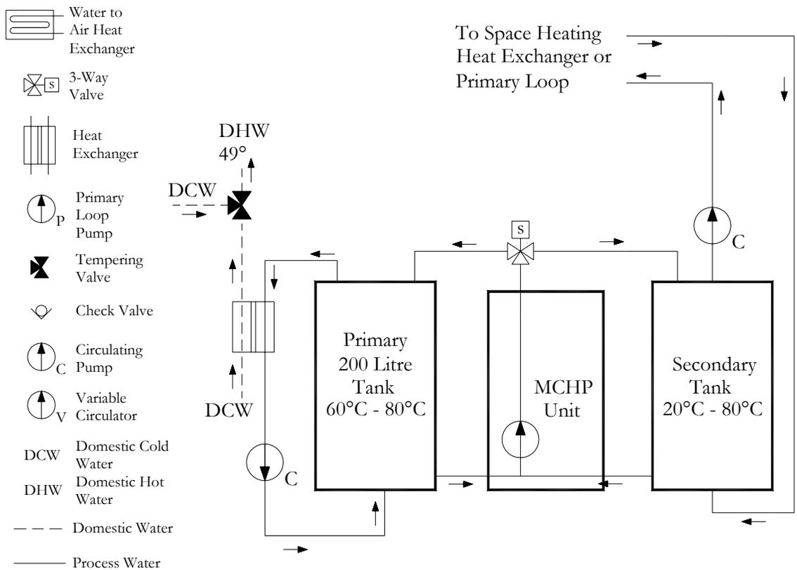
**Figure 8-2 Case F – Advanced Dual Tank Design**
