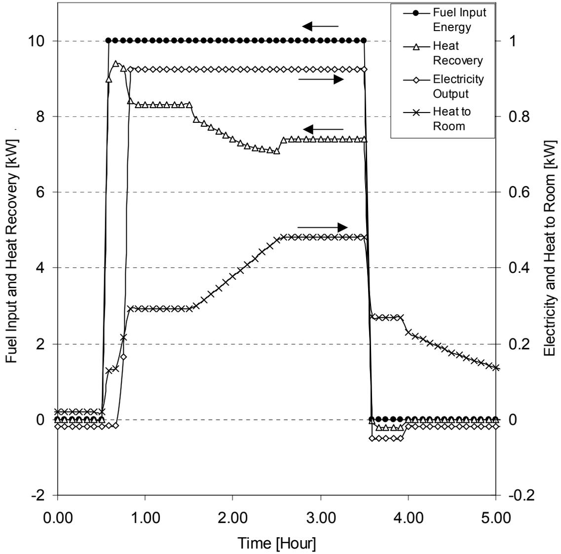
Figure 4-11 Resulting Stirling Engine Energy Flows
