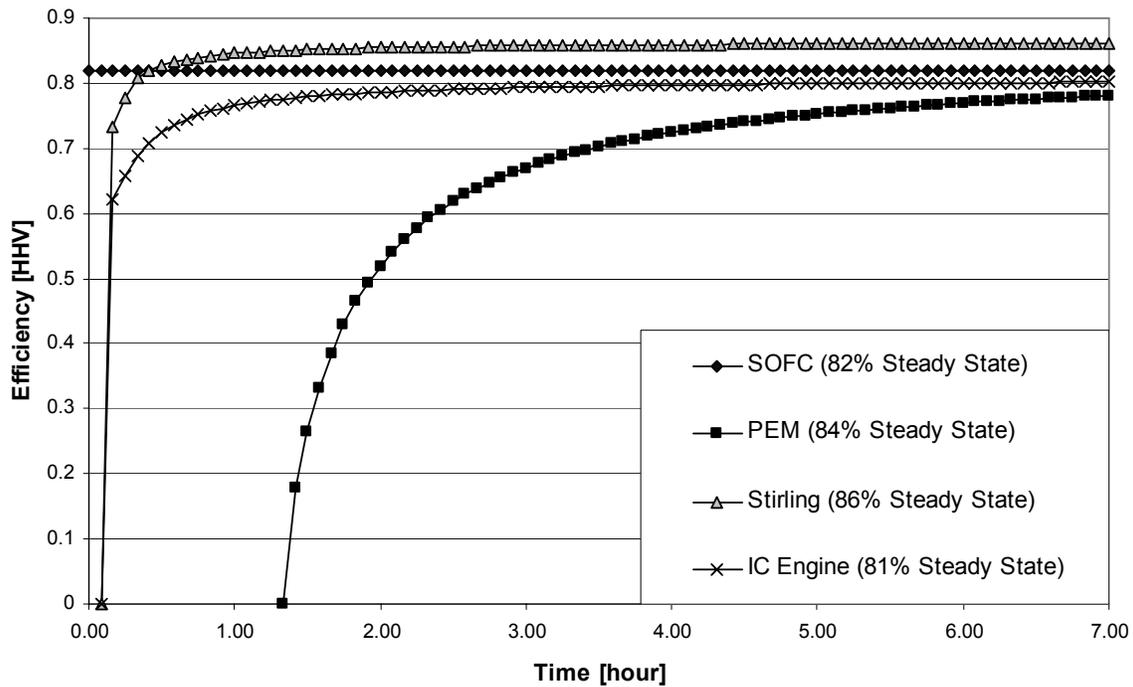
**Figure 6-2 Total On/Off Efficiency vs. Run Time (Including Cool Down Heat Recovery) – Cooling Water Inlet 40°C, Outlet 50°C**
