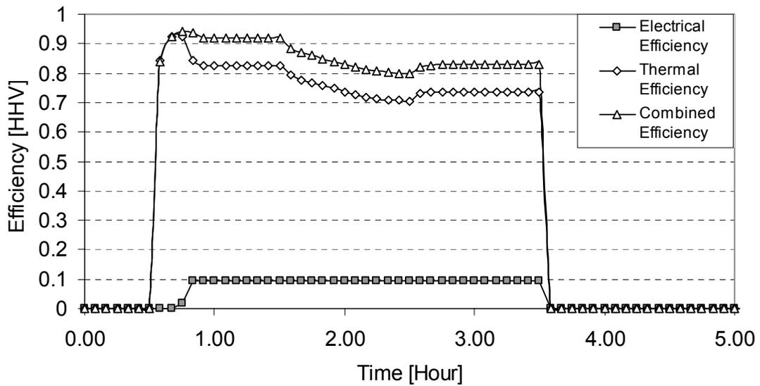
Figure 4-10 Resulting Stirling Engine Efficiencies
