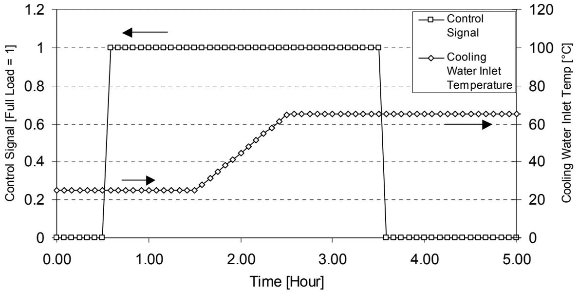
Figure 4-9 Step Input to the Stirling Engine Model – Cooling Water Flowrate at 20 Litres/min
