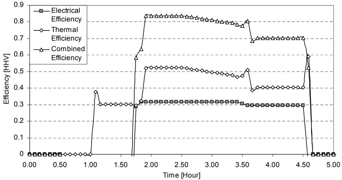
**Figure 4-7 Resulting PEMFC Efficiencies – Cooling Water Outlet Temperature Maintained at 70°C**
