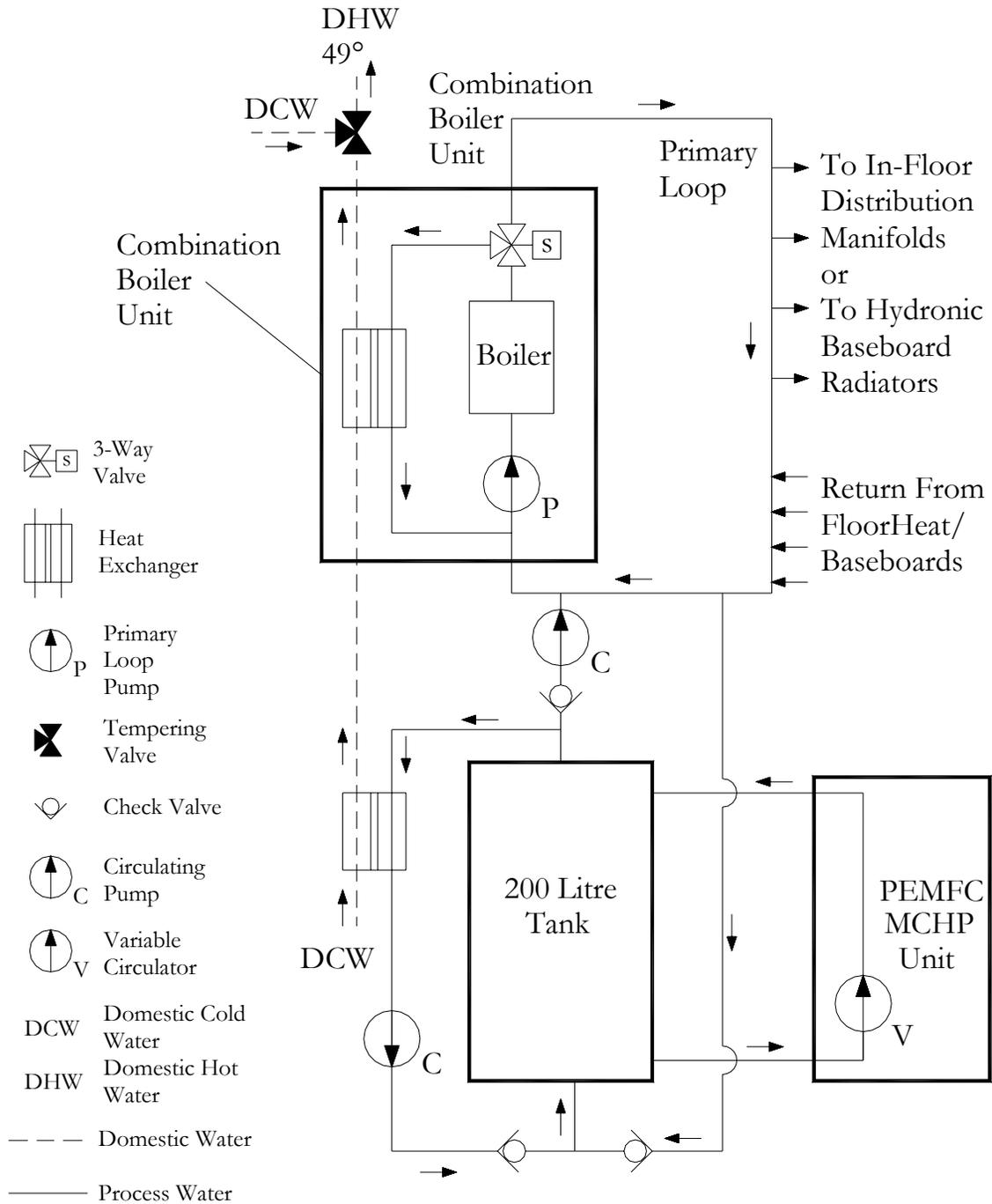
**Figure 7-6 In-Floor Heat & Hydronic Radiators / PEM Integration Cases B and C**
