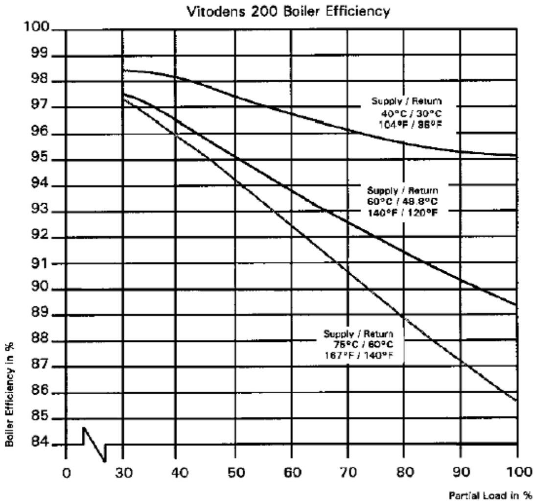
Figure 5-4 Viessmann Vitodens 200 Boiler Efficiency [49]
