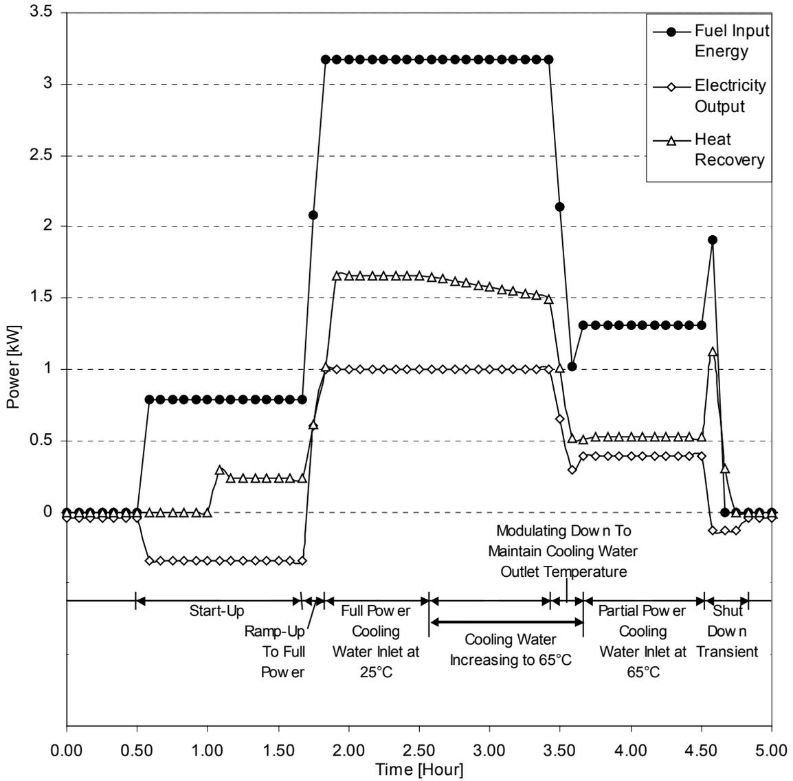
**Figure 4-6 Resulting PEMFC Transient Energy Flows - Cooling Water Outlet Temperature Maintained at 70°C**
