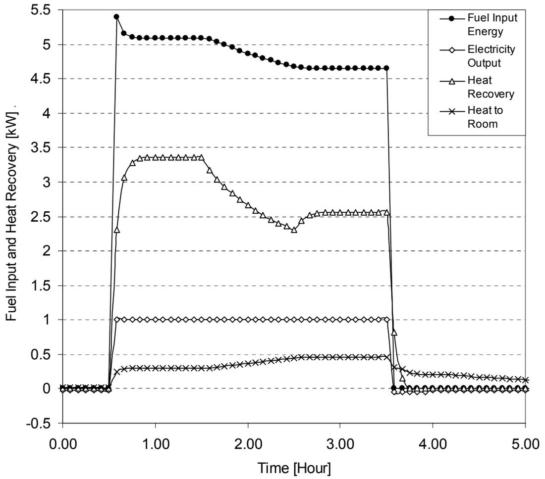
**Figure 4-14 Resulting Internal Combustion Engine Energy Flows**
