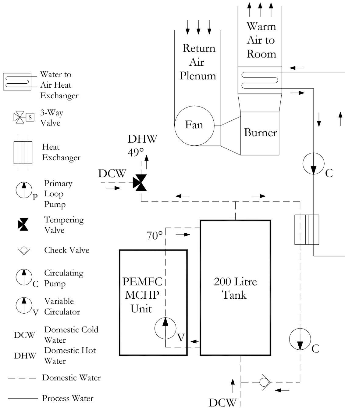
**Figure 7-4 PEM Fuel Cell / Forced Air Basic Integration**
