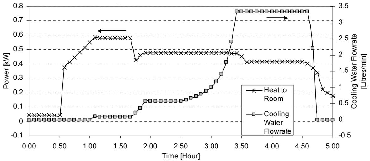
**Figure 4-8 Resulting PEMFC Heat to Room and Cooling Water Flowrate - Cooling Water Outlet Temperature Maintained at 70°C**
