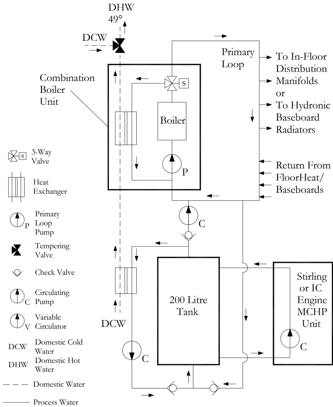
**Figure 7-8 Stirling / IC Engine In-Floor and Hydronic Radiator Heating Cases**
