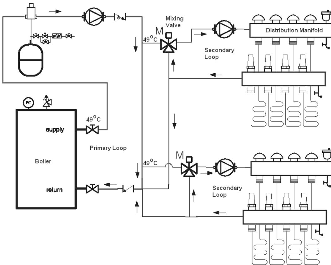
**Figure 5-1 Conventional In-Floor Heating System**
