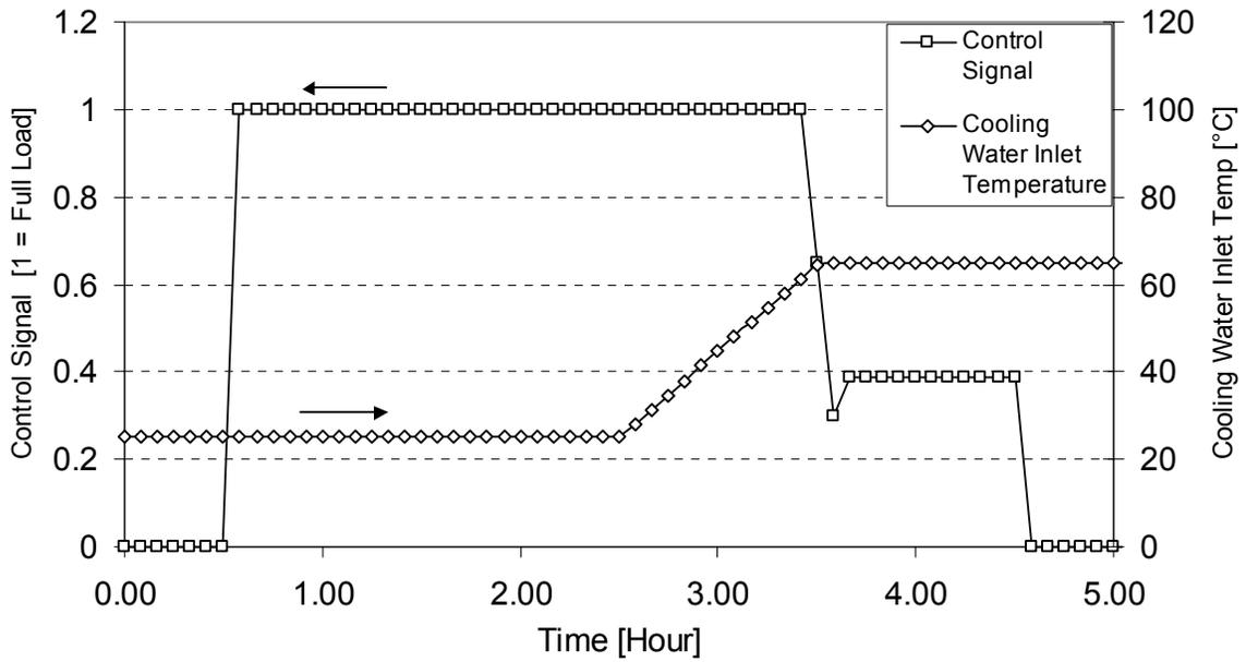
**Figure 4-5 Step Input to the PEM Fuel Cell Model - Cooling Water Outlet Temperature Maintained at 70°C**
