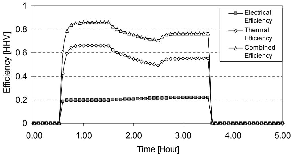
**Figure 4-13 Resulting Internal Combustion Engine Efficiencies**
