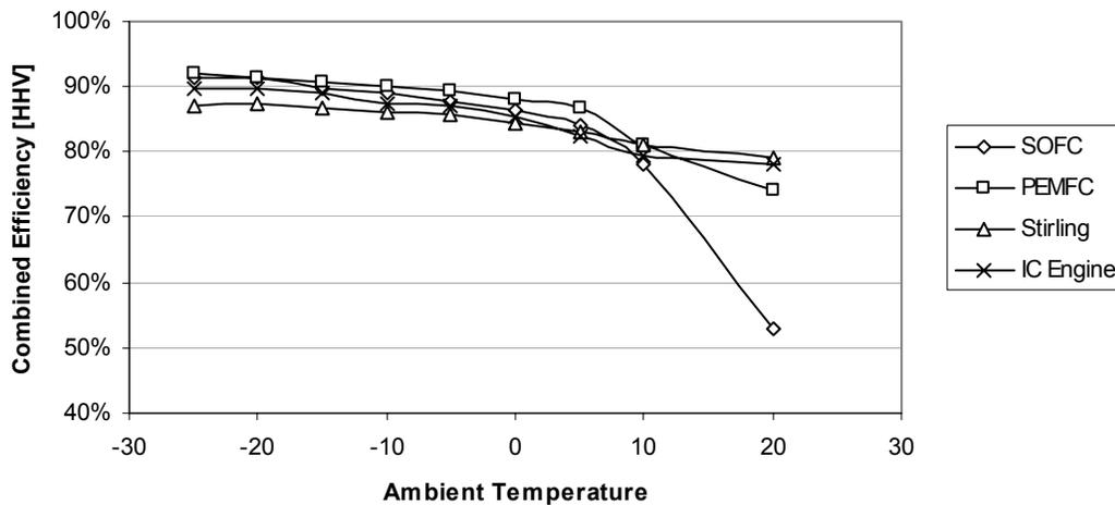
**Figure 8-3 Typical MCHP Efficiency vs. Outdoor Temperature: Advanced Integration (Excluding Ambient Skin Loss)**
