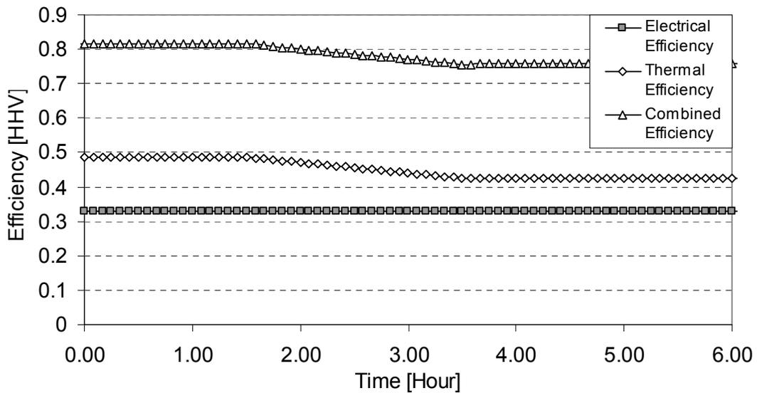
**Figure 4-3 Resulting Solid Oxide Fuel Cell Efficiencies - Cooling Water Outlet Temperature Maintained at 70°C**
