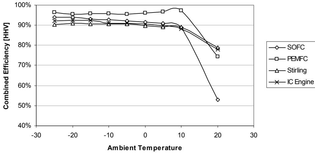
**Figure 8-4 Typical MCHP Efficiency vs. Outdoor Temperature: Advanced Integration (Including Skin Loss)**
