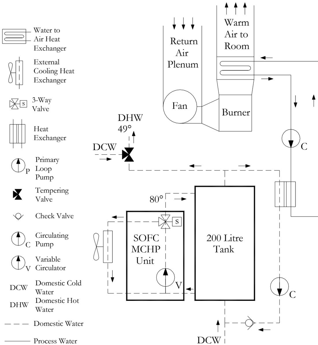
**Figure 7-1 SOFC / Forced Air Basic Integration Case "A"**
