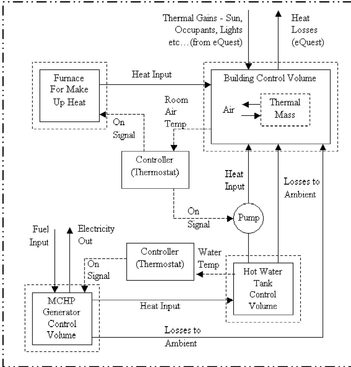
Figure A1 – Simplified Illustration of TRNSYS Simulation Software Architecture
