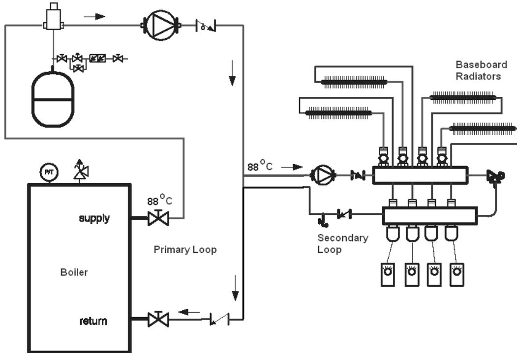
Figure 5-2 Conventional Hydronic Radiator Heating System
