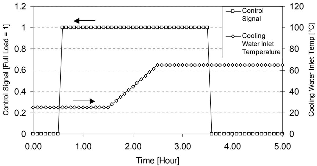
**Figure 4-12 Step Input to the Internal Combustion Model – Cooling Water Flowrate at 6 litres/min**
