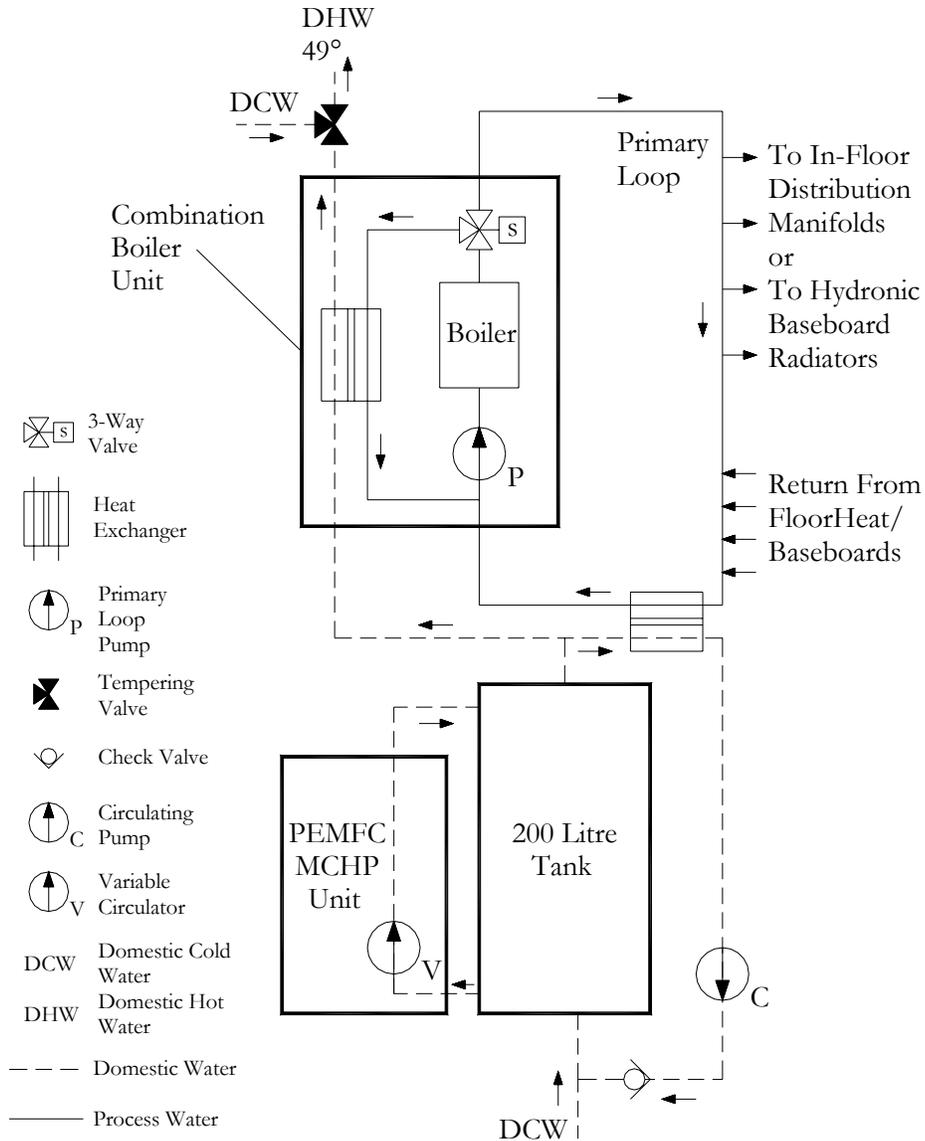
**Figure 7-5 In-Floor Heat & Hydronic Radiators / PEM Integration Case A**
