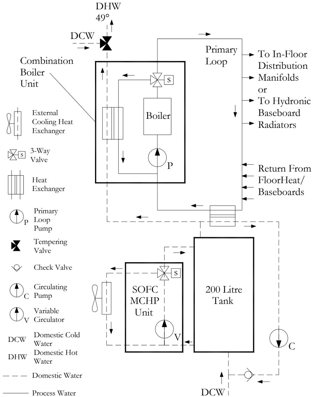
**Figure 7-2 SOFC / In-Floor and Hydronic Radiator Heating Case A**
