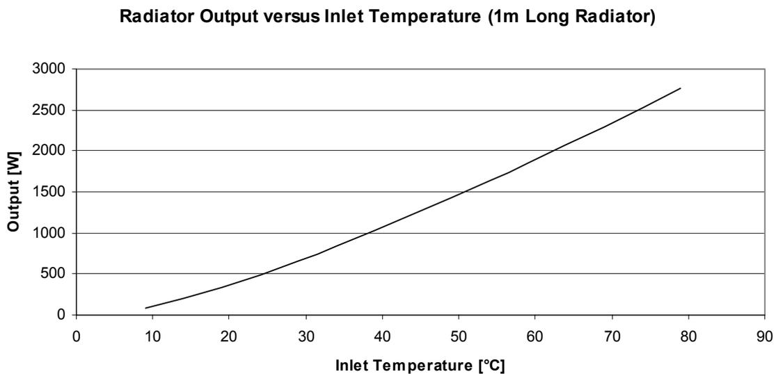
**Figure 5-3 Baseboard Heat Output vs. Inlet Water Temperature (1m long radiator)**
