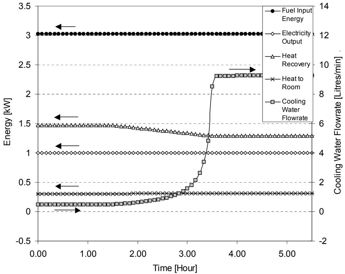
**Figure 4-4 Resulting Solid Oxide Fuel Cell Energy Flows - Cooling Water Outlet Temperature Maintained at 70°C**
