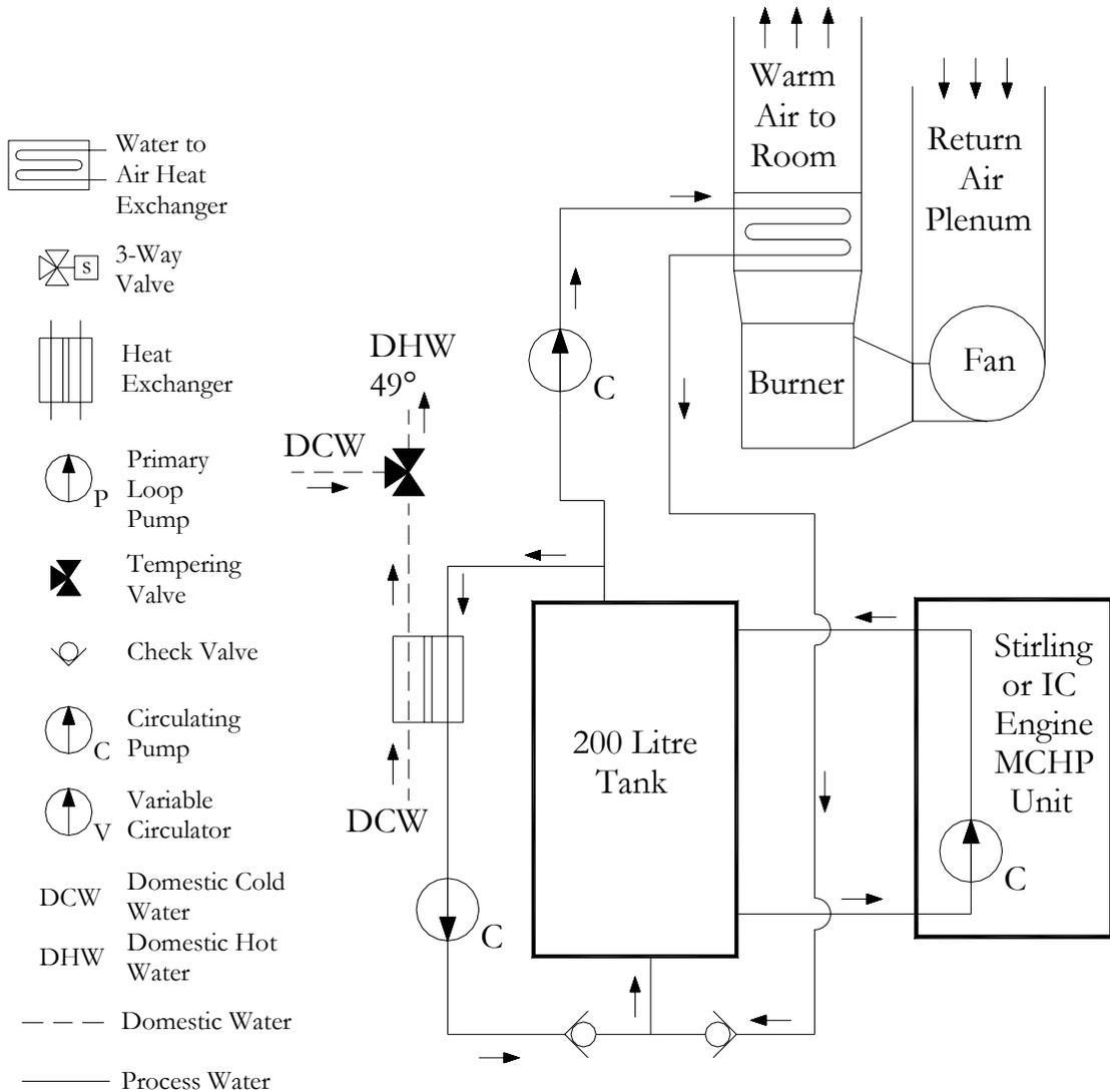
Figure 7-7 Stirling and IC Engine Basic Forced Air Integration
