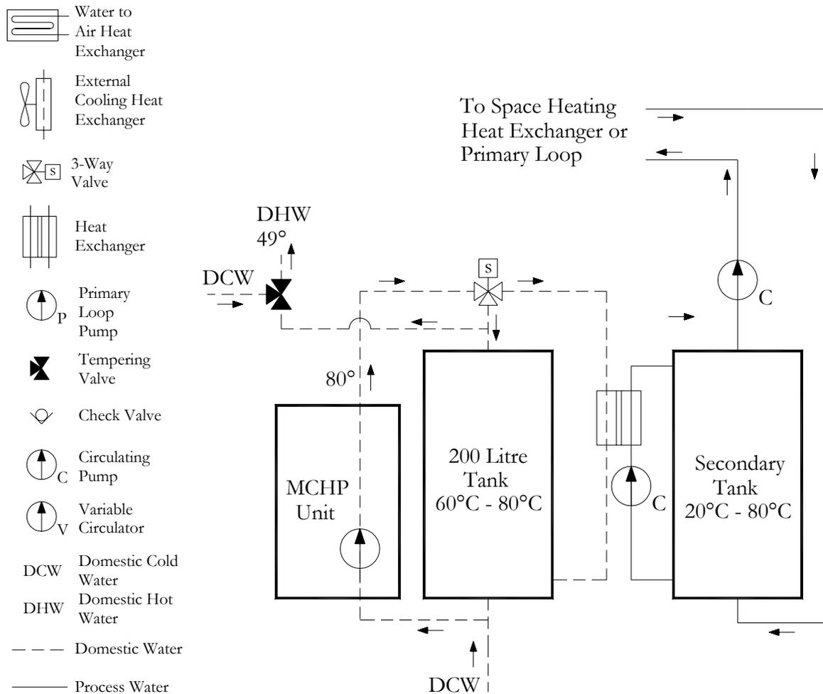
**Figure 8-1 Case E – Dual Tank Design**
