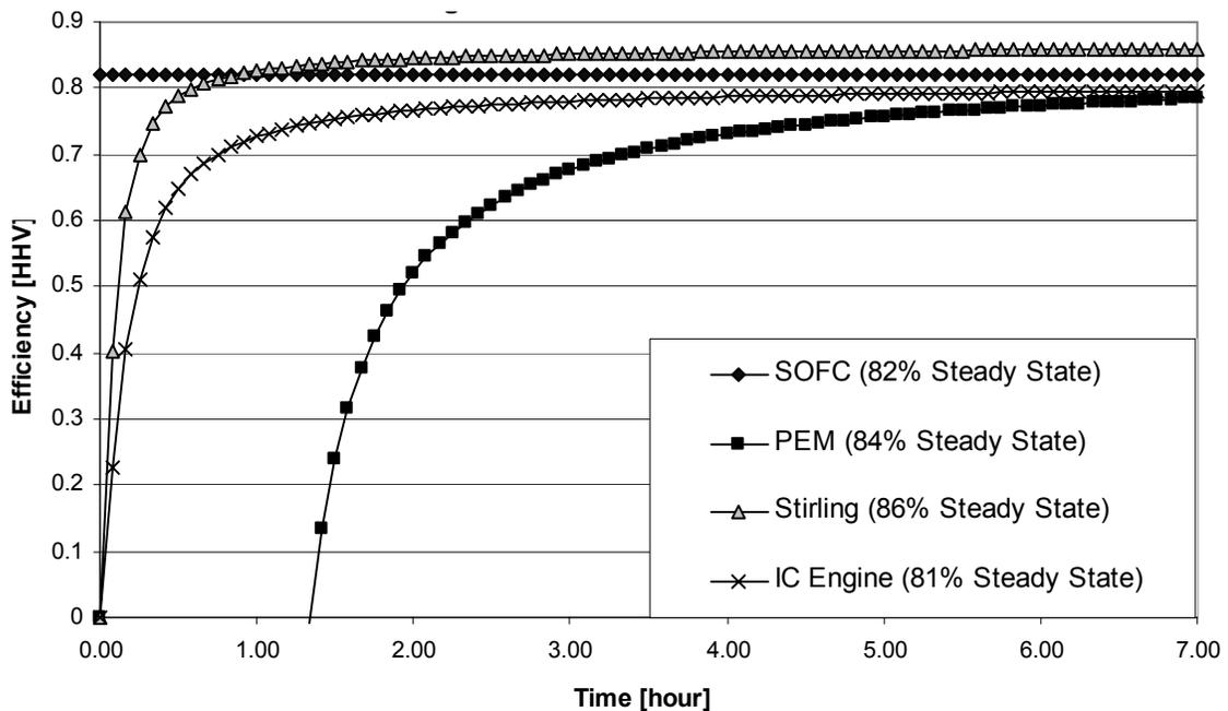
**Figure 6-1 Cumulative Efficiency With Respect to Length of Run Time – Cooling Water Inlet 40°C, Outlet 50°C**
