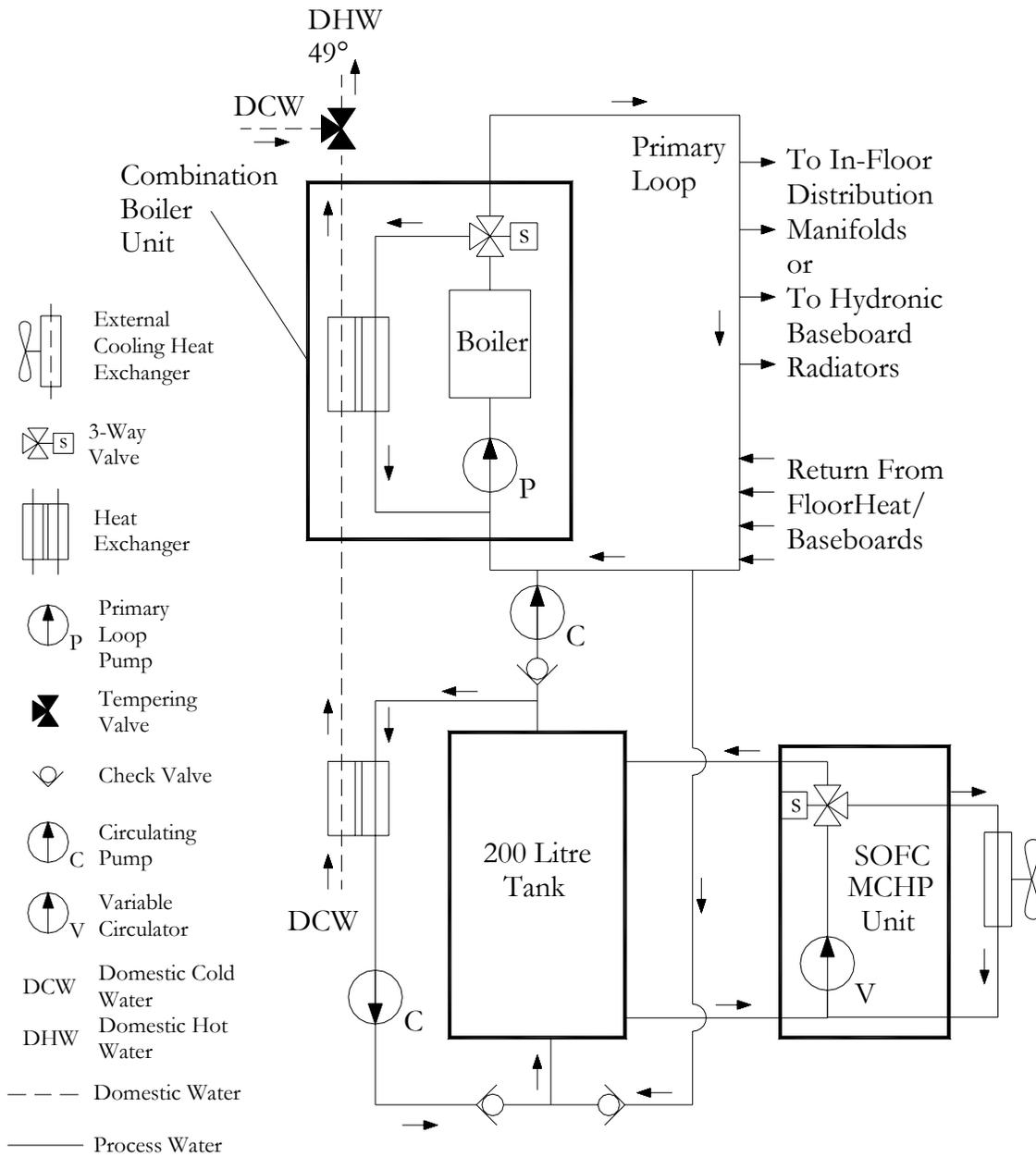
**Figure 7-3 SOFC / In-Floor and Hydronic Radiator Heating Case B and C**
