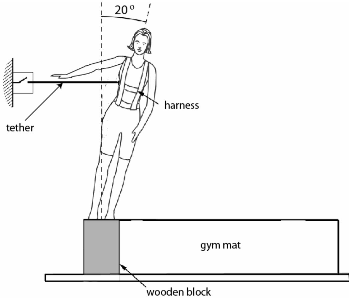
**Figure 2-1 Experimental setup.** A sideways fall was unexpectedly initiated by releasing a tether, which held the subject at a 20° lean angle.
