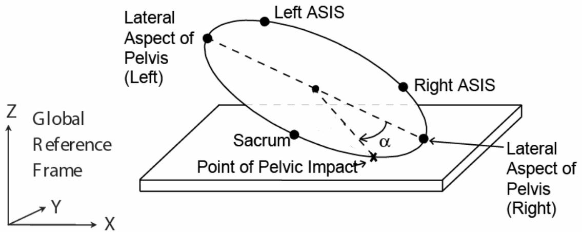
**Figure 2-2 Definition of hip proximity angle.** The hip proximity angle, which is shown by alpha in the diagram, is an absolute angle that reflects how near the site of pelvis impact is to the lateral aspect of the hip. An angle of 0 degrees indicates direct impact to the lateral aspect to the hip, while +90 degrees reflects impact to the anterior aspect of the pelvis and -90 degrees indicates impact to the posterior aspect of the pelvis.
