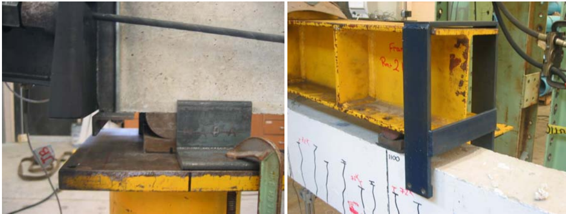
Figure 4.19: (a) Steel angles located at the beam edges and (b) the restraint system for spreader beam
