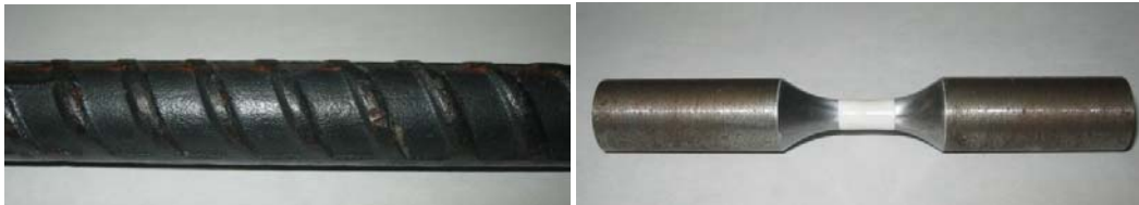
Figure 5.22: (a) Deformed rebar and (b) standard machined fatigue specimen
