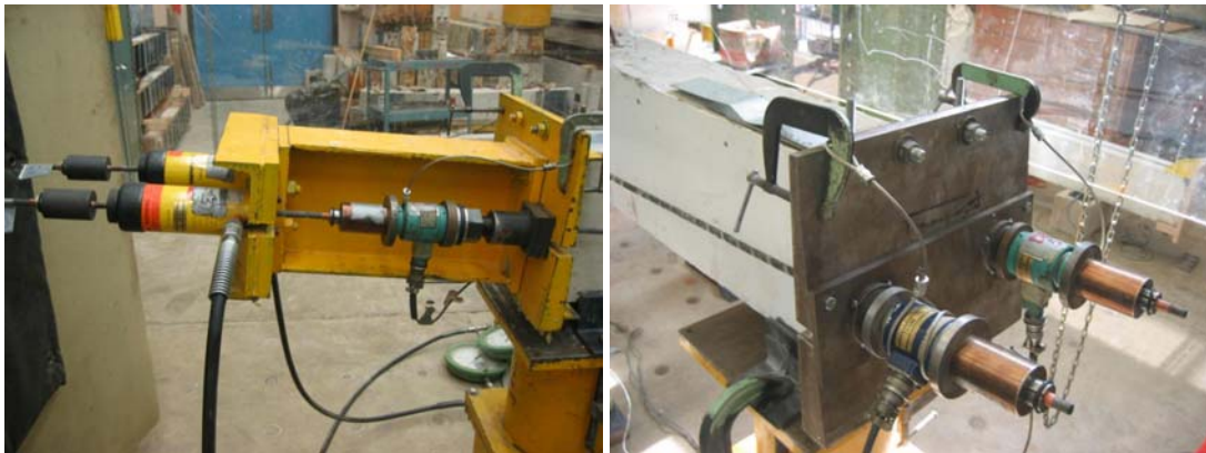
Figure 4.11: General view of the jacking end (left) and the dead end (right) of the end-bearing system
