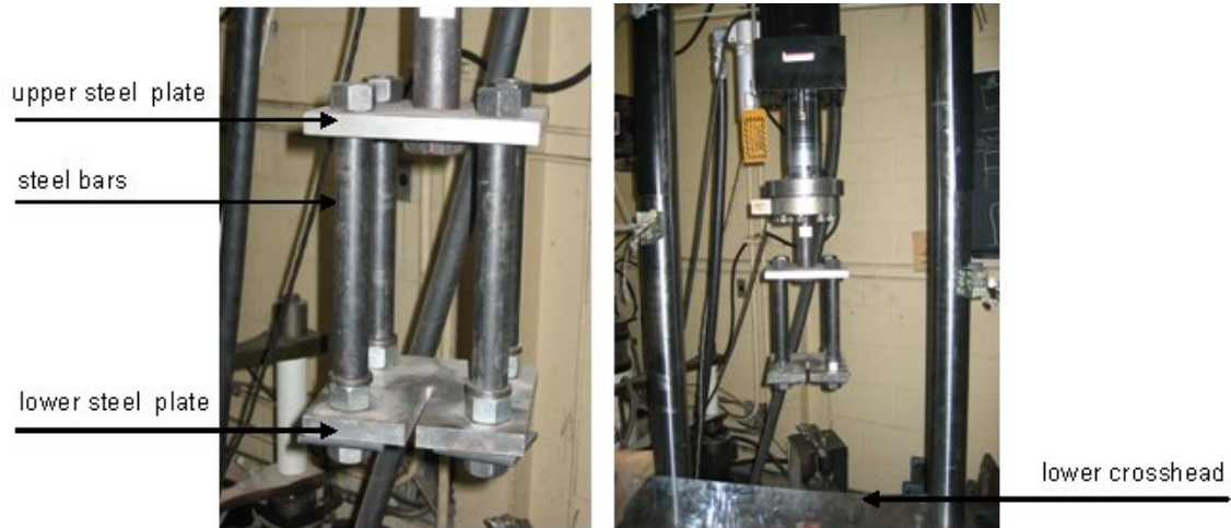
Figure 3.4: Test rig attached to the actuator
