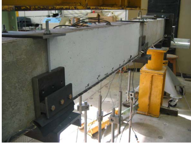
Figure 4.5: General view of a strengthened beam with straight tendon profile
