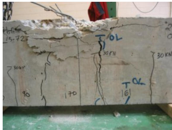
Figure 5.35: Failure of the beam OL15-F72-a by concrete crushing
