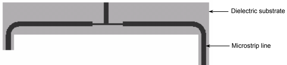
Fig. 5.33 Schematic of the designed microstrip-line junction using the high-K ceramic substrate (top view).
