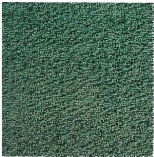
Omnicrot 7V27U Tufted, slit-film polypropylene (urethane backing) face weight 27 oz tennis Stadia Turf Systems
