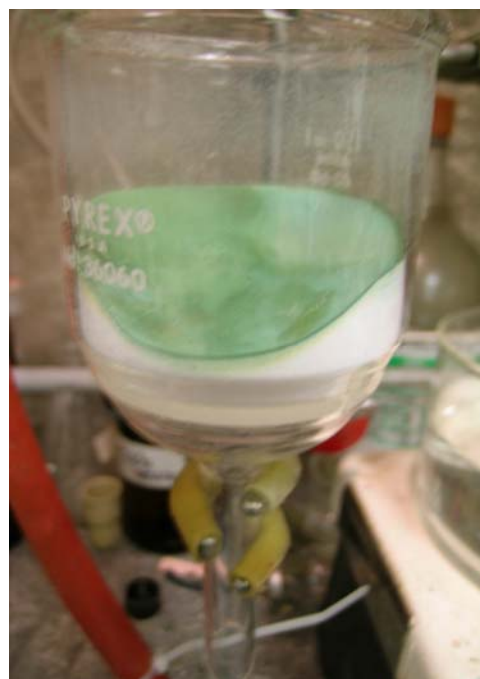
Figure 3.2 Aluminium oxide after filtering the polymer solution. The green color is caused by the presence of \text{CuBr(II)} .
