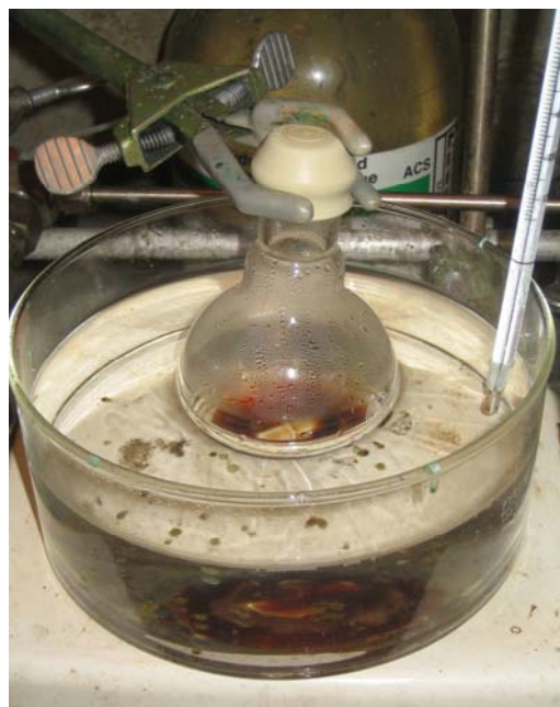
Figure 3.1 Picture of the reaction mixture in the reactor during the polymerization. The brown colour is caused by the presence of \text{CuBr(I)} .
