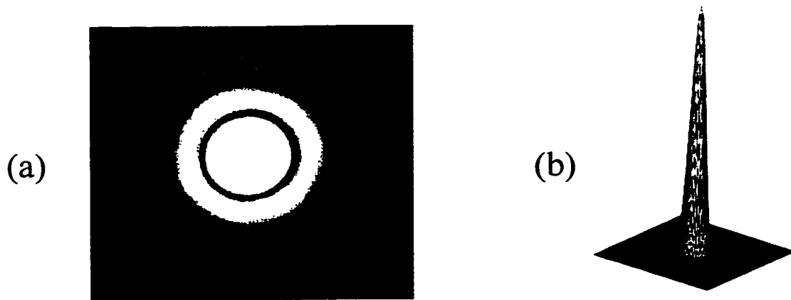
Figure 5.2 (a) The Airy disk. The central spot has been overexposed in order to make visible the surrounding disks. (b) The Airy disk pattern shown in 3D where height represents intensity. The maximum intensity on the first ring represents only 1.75% the intensity for the central peak. Figures modified from Hecht 4 .
