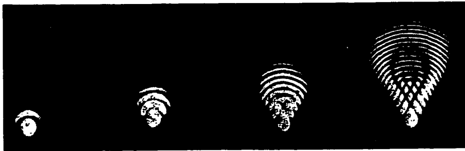
Figure 5.7 The effect of coma on the Airy disk. Figure modified from Born and Wolf 6 .
