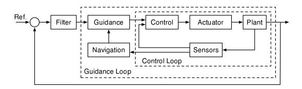
Figure 4.1: A typical guidance, navigation, and control system
