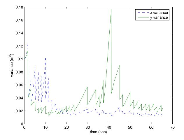
Figure 5.9: Straight line test: **x** and **y** variance
