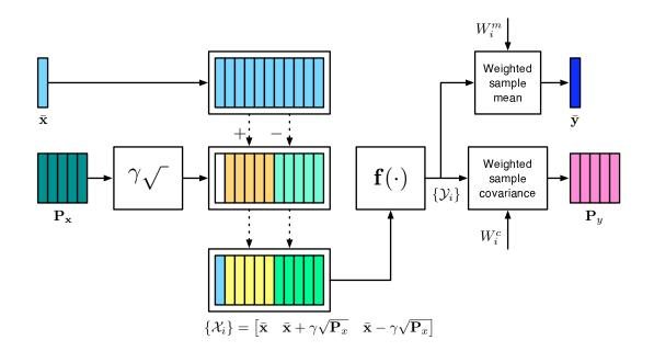
Figure 3.2: UT block diagram
