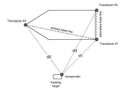
Figure 5.6: Target position determined by "Short Baseline" method
