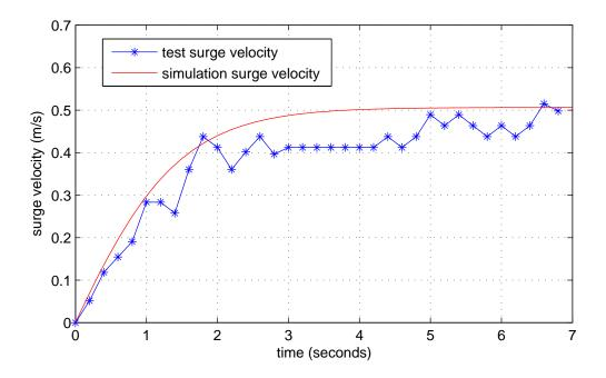
Figure 2.13: Surge test experiment data and simulation result
