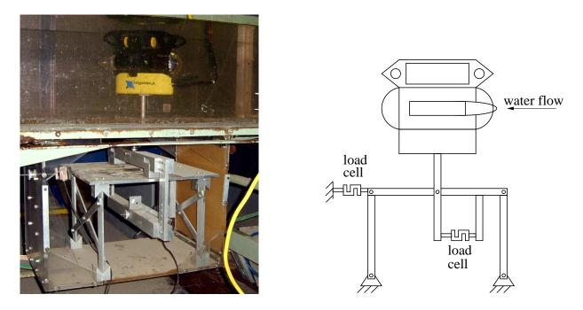
Figure 2.3: horizontal-bending mechanism in the flume test
