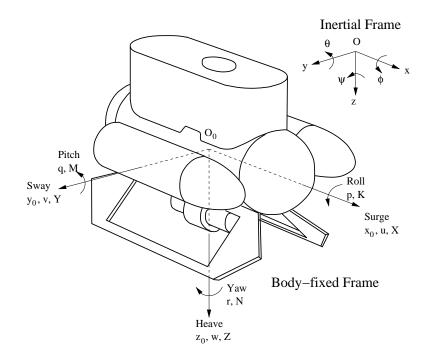
Figure 2.2: Body-fixed and inertial reference frames
