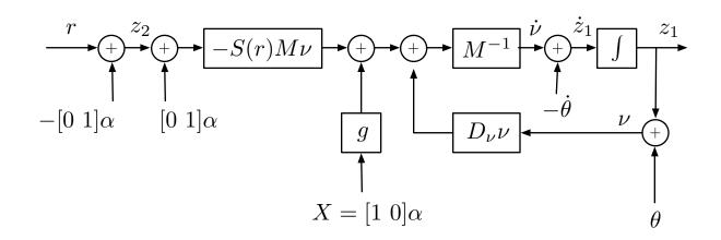
Figure 4.6: After backstepping for  $z_1$
