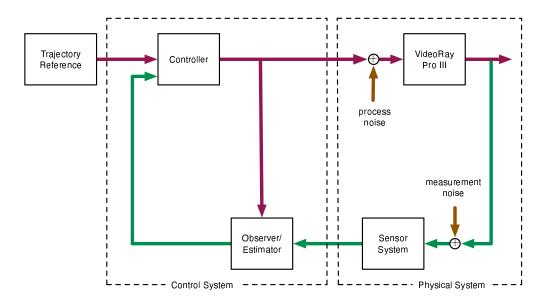
Figure 1.4: Autonomous control system configuration
