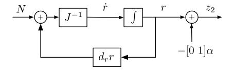
Figure 4.7: Before backstepping for  $z_2$
