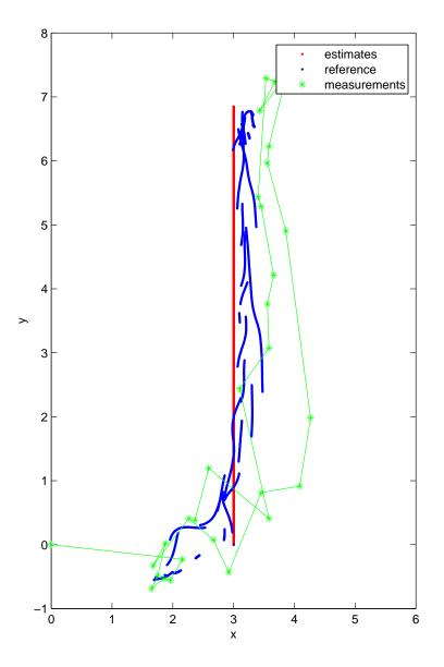
Figure 5.8: Straight line test trajectory: The reference trajectory is a straightline starting from (3, 0) to (3, 7.8) and then returning back along the same line to the starting point; The green asterisks show the Pilot measurements as the vehicle is moving along the trajectory. The blue line segments show the estimates of the vehicle's position achieved through the UKF.
