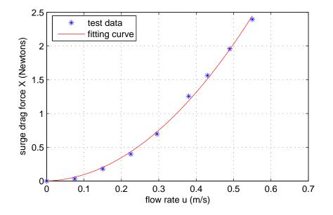
Figure 2.6: Drag force in surge direction: experiment data and fit curve
