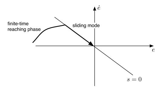
Figure 4.9: Graphical interpretation of sliding surface
