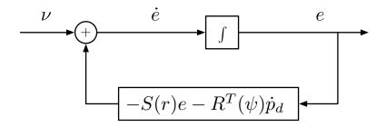
Figure 4.3: Block diagram for error dynamics  $\dot{e}$
