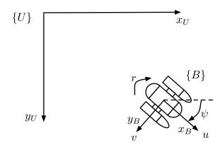
Figure 4.2: Body-fixed  $\{B\}$  and earth-fixed  $\{U\}$  coordinate frames
