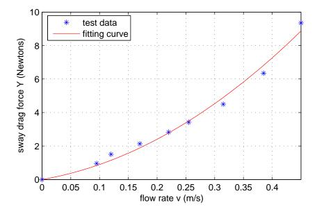
Figure 2.7: Drag force in sway direction: experiment data and fit curve
