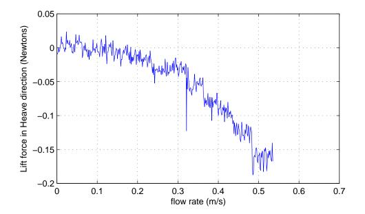
Figure 2.9: Heave lift force vs. surge speed
