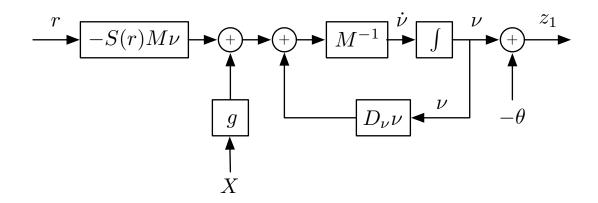
Figure 4.5: Before backstepping for  $z_1$
