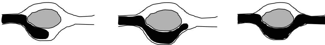
Figure 2.10 Drainage displacement mechanism in pore doublet [after Chatzis et. al. 1983].
