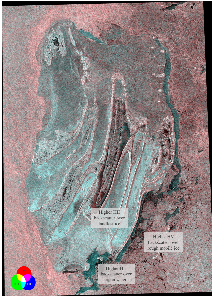
Figure 2.3: Sentinel-1 SAR image ( \sigma^0 dB) acquired May 5, 2016, over the Belcher Islands in Hudson Bay. Composited as (R=HV, G=HH, B=HH), with each band clipped to (0.5, 99.5) percentiles. Annotations indicate different sensitivities of HH and HV backscatter intensity to ice types and open water. Relatively high HH backscatter over smooth landfast ice in this image may reflect a brine-wetted snowpack as spring air temperatures increase.
