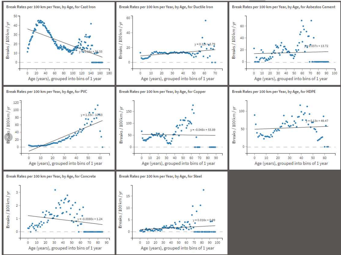
Figure 35: Break rates per 100 km per year, by age, for each material type.
