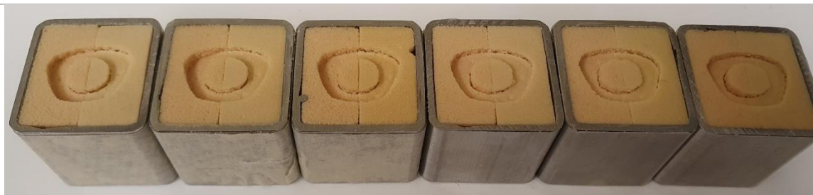
Overhead view of deformed sandwiched PU foam samples. Samples 1B, 2B, 3B, 4B, 5B, 6B using BSJ setup depicted.
