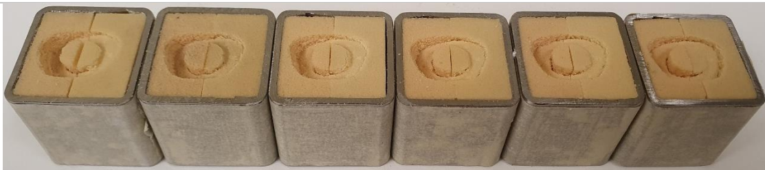
Overhead view of deformed sandwiched PU foam samples. Samples 1B, 2B, 3B, 4B, 5B, 6B using FC setup depicted.
