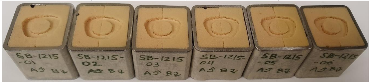
Overhead view of deformed sandwiched PU foam samples. Samples 1A, 2A, 3A, 4A, 5A, 6A using BSJ setup depicted.
