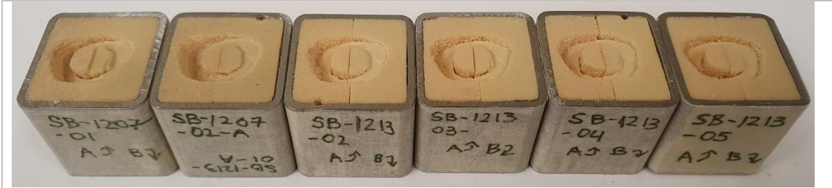
Overhead view of deformed sandwiched PU foam samples. Samples 1A, 2A, 3A, 4A, 5A, 6A using FC setup depicted.
