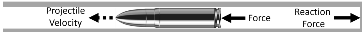
Figure 1: Projectile propulsion through the barrel and the recoil force applied over the LPR. Adapted from (Hazell, 2021)
