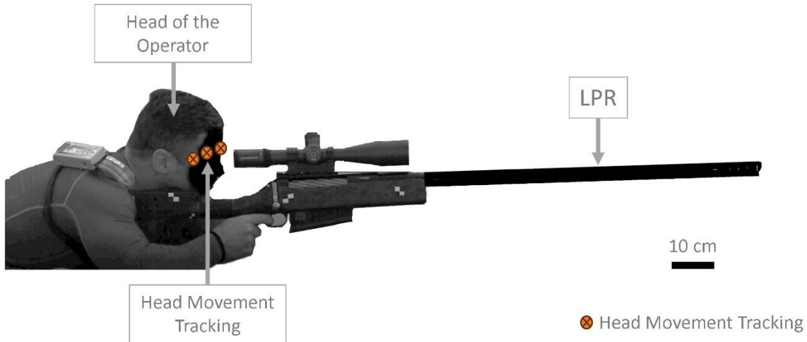
Figure 18: The operator in a prone position discharged an LPR with a suppressor configuration, and the head movement was tracked using tape marks and free-source video tracking software.
