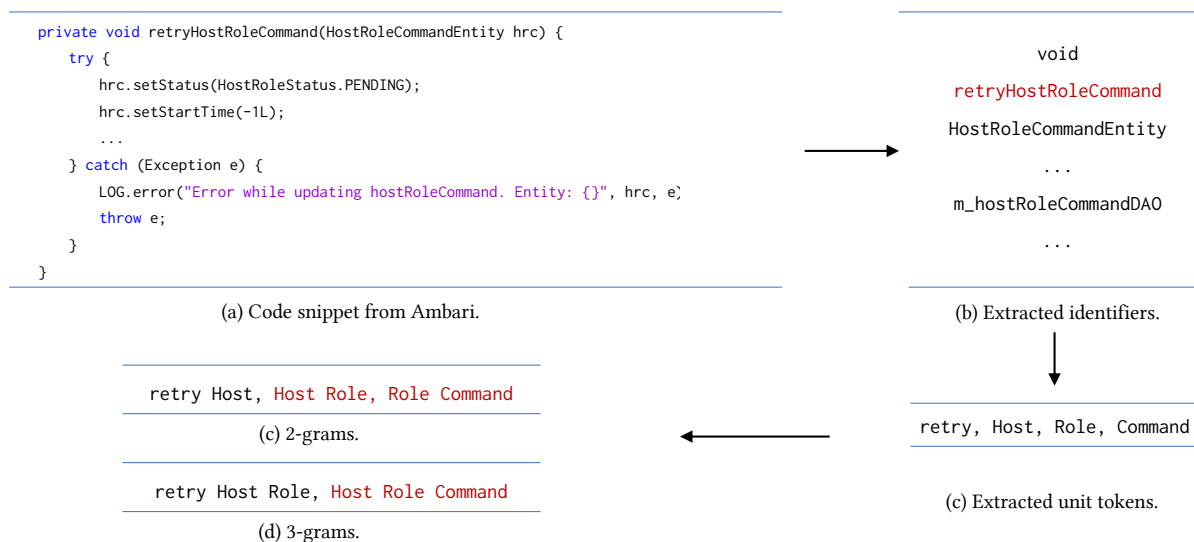
Figure 6.10: An overview of the process of building n -gram dictionaries from the source code.
