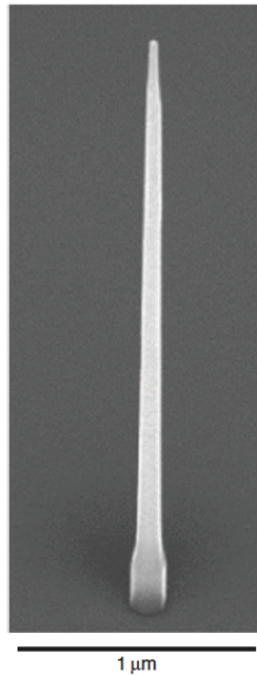
Figure 2.8: Scanning electron microscope of a tapered nanowire waveguide with a QD embedded 200 nm from the base of the wire [2].
