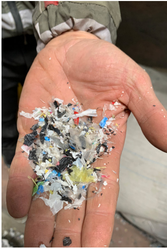
Fig.4.17 Shredded dry plastics to be fed into another machine for processing. Photographed by author in Manshiyat Nasser
