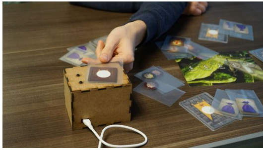
(a) Player using the Leader Token that is embedded with an NFC sticker
