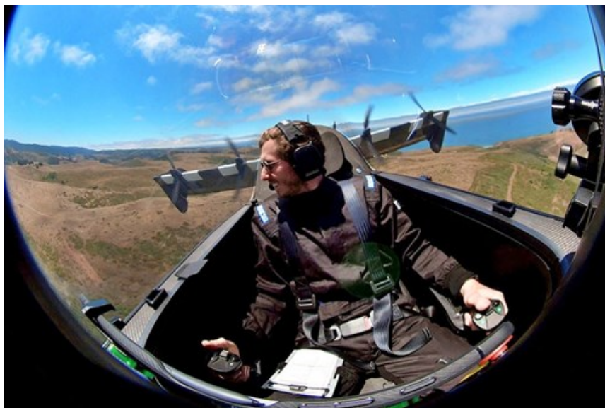
Figure 2.10: The pilot inside the BlackFly is using the joysticks to pilot the aircraft [23].
