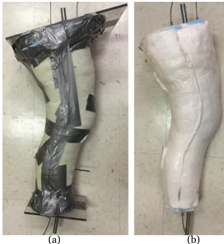
Figure 4.7: (a) Sample specimen contained within its sealed negative mould; and (b) the ‘foamed’ specimen with hip, ankle attachment rods and three muscle force cables.
