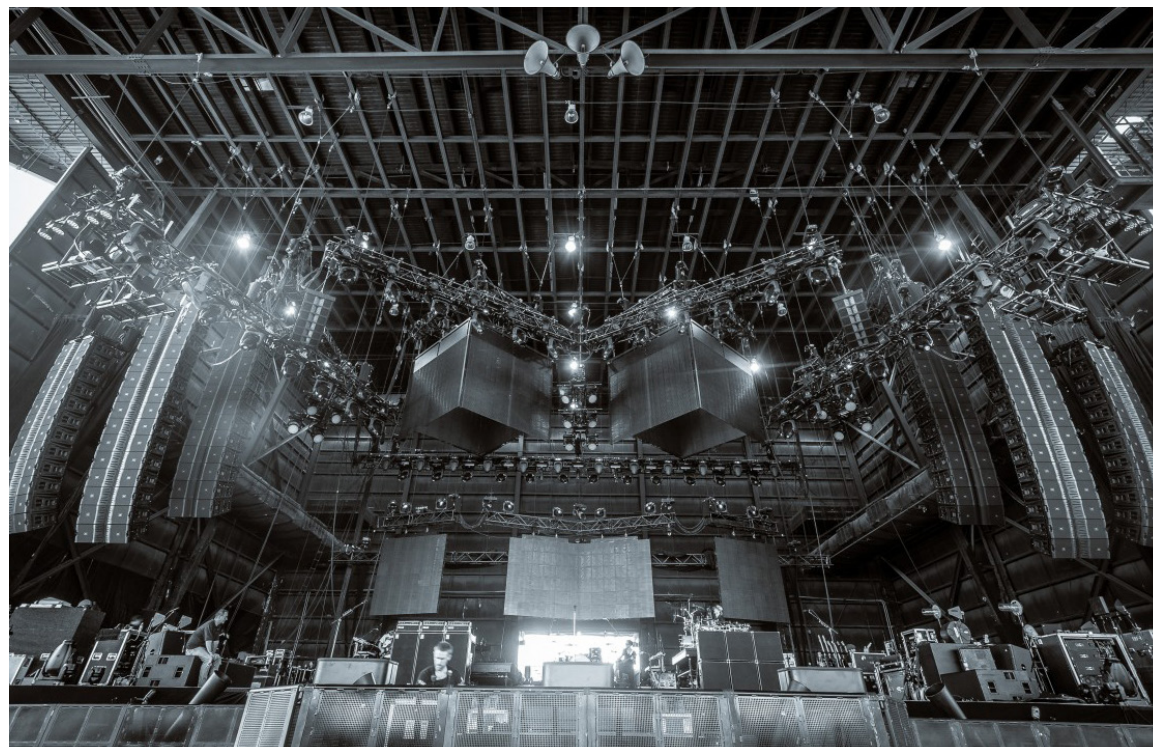
fig. 16: Showing the placement of speakers within the overall spatial layout of a typical arena sized concert. These can change slightly depending on the arena size but will usually follow this pattern.
