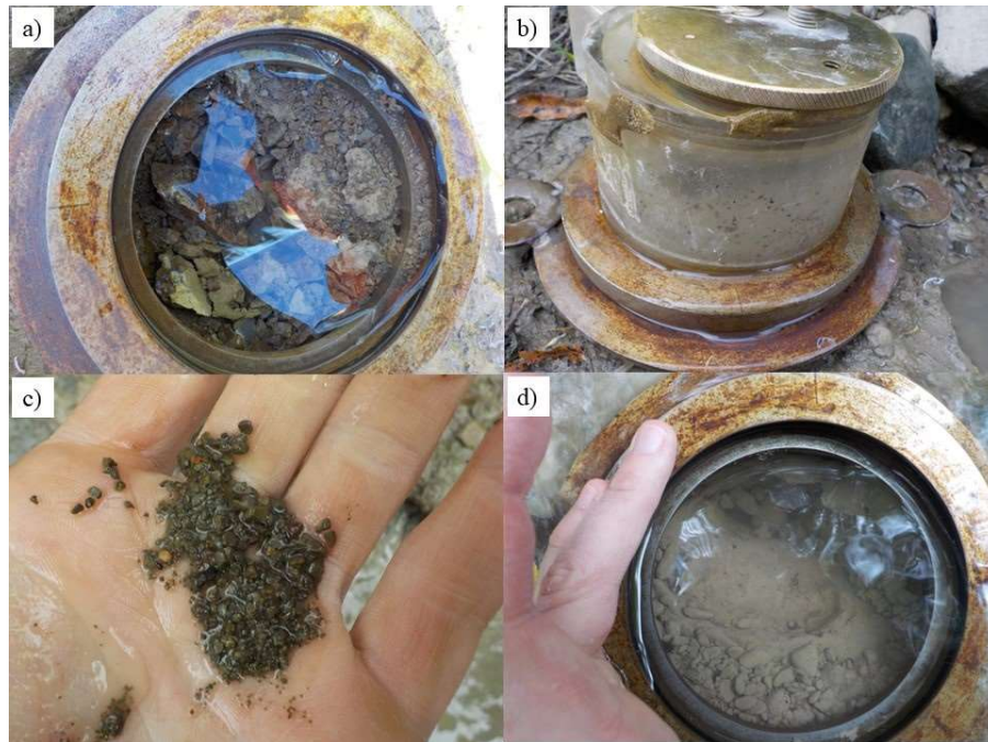
Figure 5: Factors influencing the representativeness of JET. a) fracturing and block separation at Whirl Creek, b) sands causing abrasion during test at MCE, c) sands retrieved from scour hole at FC, d) Maximum scour not aligning with measuring point at NTL.
