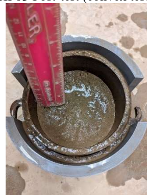
CCT9-HP02-MJC2 Post-Test (Flat Test Surface)
