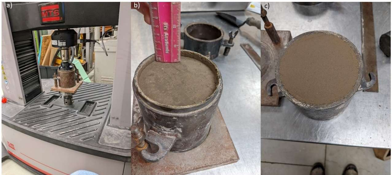
Figure G1: a) sample consolidation using EM press. b) reduction in sample height after consolidation. c) bottom of prepared sample which was used as test surface
