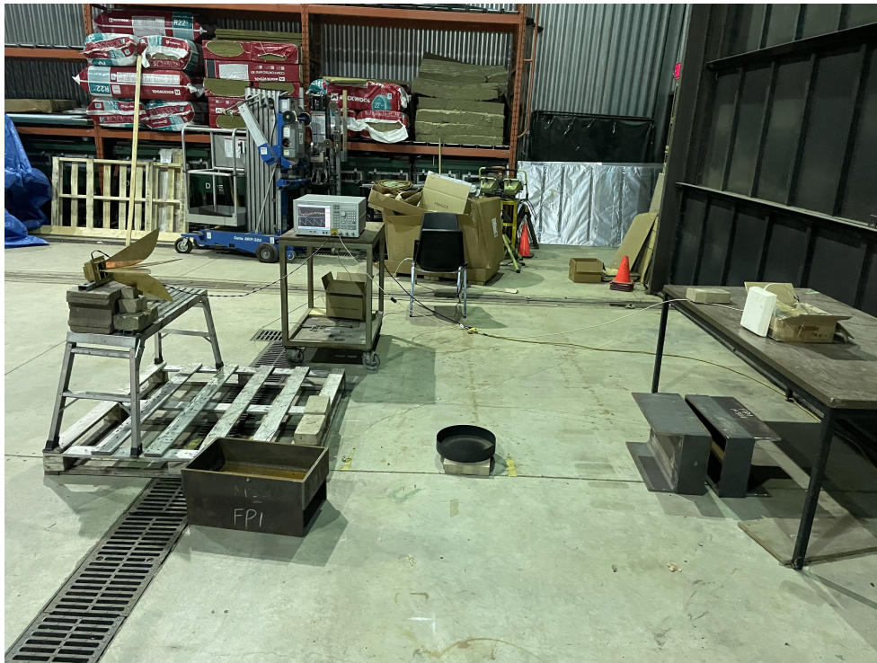
Figure 3.11: Photo of heptane smoke experiment setup. The hardware setup is the same as the longer-range experiment in Figure 3.8 except that the metal pan is placed on the floor.
