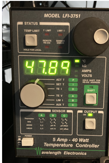
Figure 3.16: Photograph of the temperature controller for the doubler for the 1107 nm laser. Emitted light frequency stability depends on the stability of the doubler temperature.
