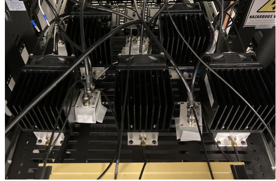
(b) AOM RF drive circuit drawer 2.
