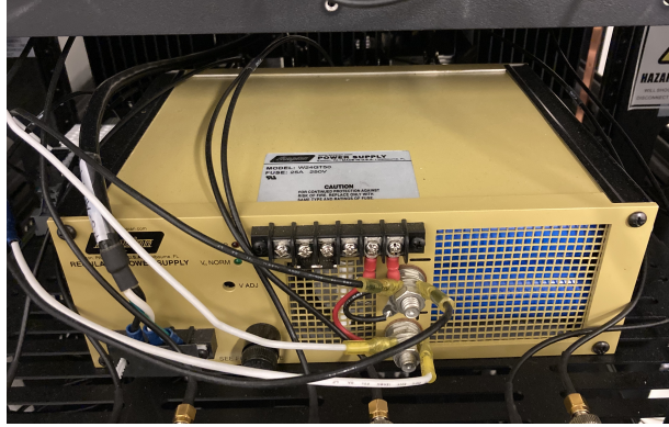
Figure 3.6: The PSU for the trap RF drive circuit power amplifier. The same PSU also supplies power for the AOM RF drive circuit power amplifiers (Section 3.2.4).
