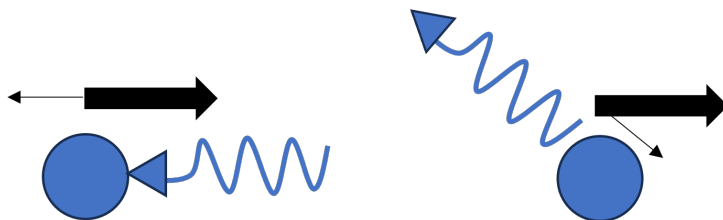
Figure 2.9: Diagram of a photon scattering from an atom (not to scale). Left: when the atom absorbs the photon, its momentum changes. Right: when the atom emits the photon, its momentum changes as well. Since the direction of photon emission is random, the net change of momentum due to photon emission averages to zero, while the change in momentum due to preferential absorption of photons from a single direction may be significant. The black arrows represent the momentum of the atom, with the large arrow indicating the motion of direction of the atom and the small vector showing the change of momentum due to scattering events with the photon.
