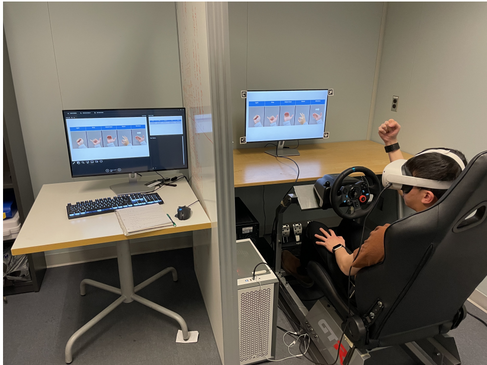
Figure 3.9: Wizard-of-Oz experiment room setup, the researcher sits on the left side of the board to operate the features, while the user sits on the right side of the board
