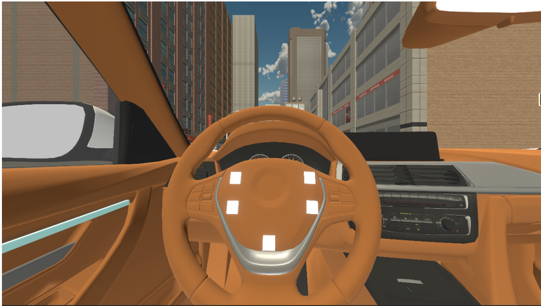
Figure 3.3: Steering wheel in Virtual environment (white blocks for better participants' button recognition). The position is aligned with the real steering wheel
