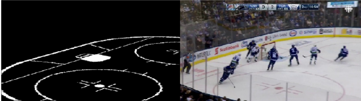
Figure 3.3: In this case, the overhead template is warped using the result of the initial estimator module, to produce the warped template seen on the left. The refinement module takes the warped template and the actual video frame, and tries to calculate the homography needed to warp between the two using the 4-point approach.
