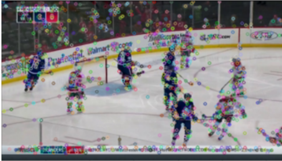
Figure 2.3: SIFT [27] features on a hockey broadcast frame. Unfortunately, the vast majority of detected features do not relate to rink features.
