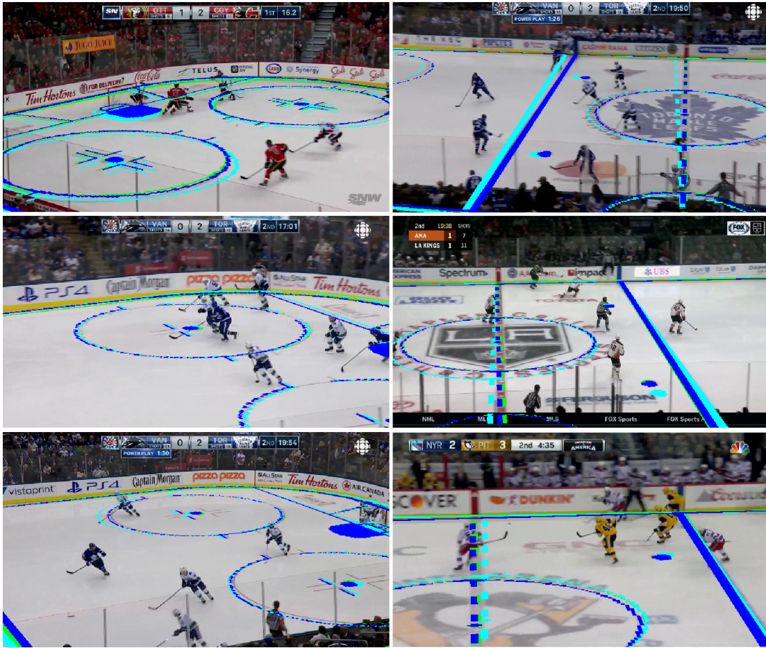
Figure 4.15: Example results on NHL validation data. Green is ground truth, light blue is initial homography estimate, and dark blue is the final homography after refinement. Note that sometimes the green may be covered completely by the blue at points due to how the results are visualized.
