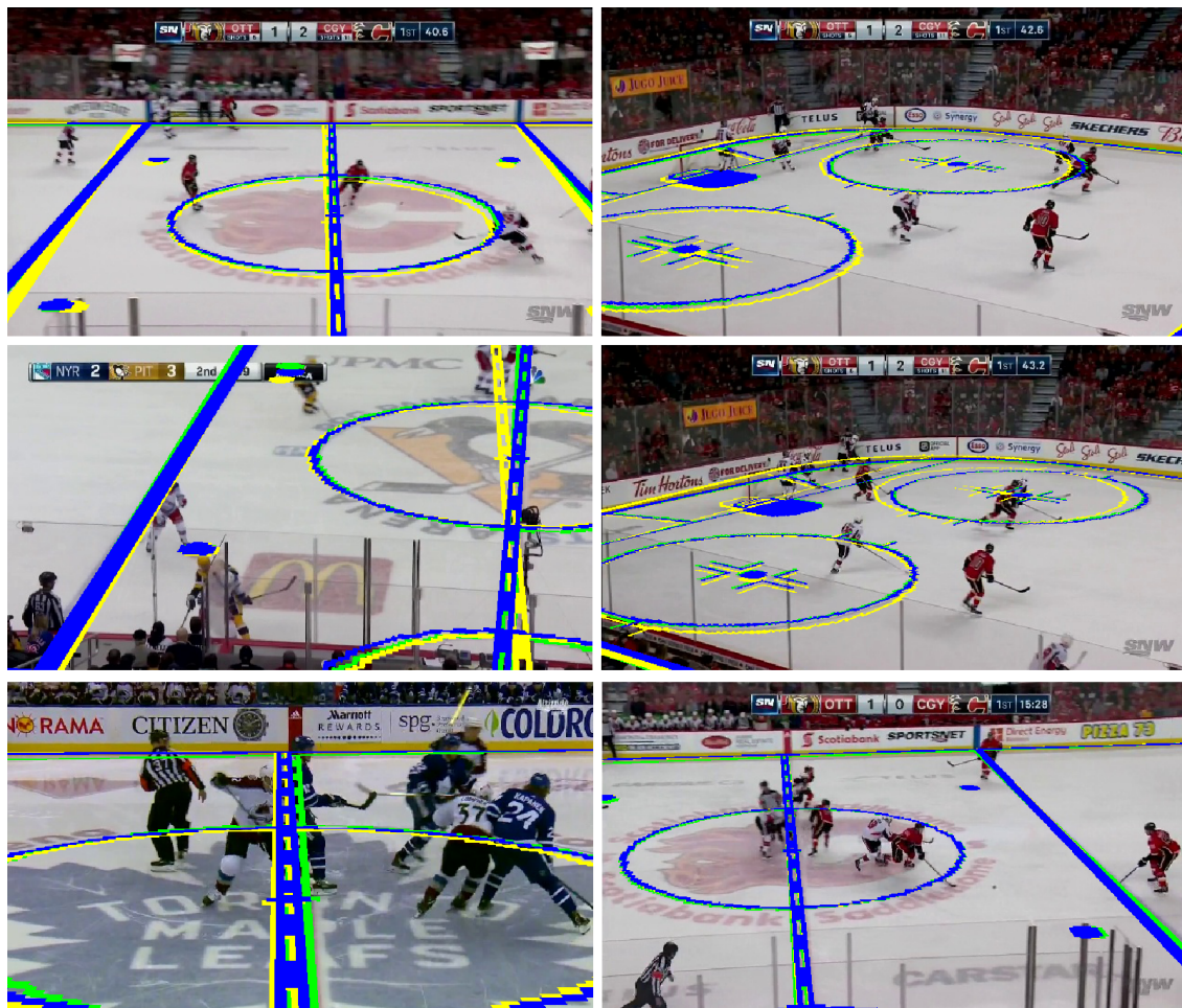
Figure 3.9: Examples of homography results. The green lines represent ground truth, the yellow lines represent the initial estimator result, and the blue lines represent the refined estimate result. Bottom row shows a couple of cases where lines are still not aligned even after refinement.
