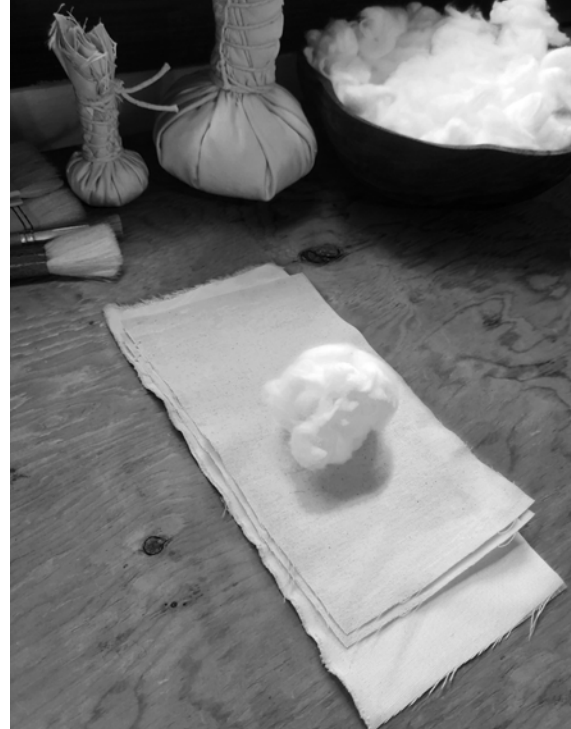
Fig. 3.3 Photograph of the layered pieces of silk and cotton cloth during dabber construction by the author.
