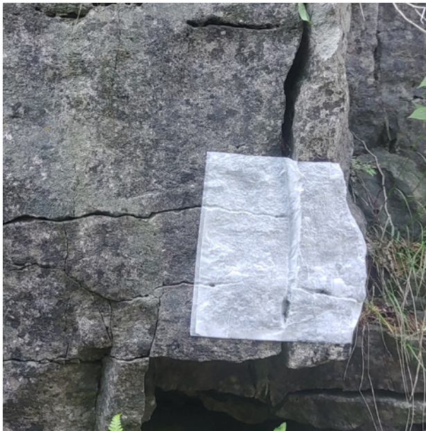
Fig. 3.16 Photograph of wetted and tamped sheets of paper on the cliff face of the Niagara Escarpment during a site visit by the author.
