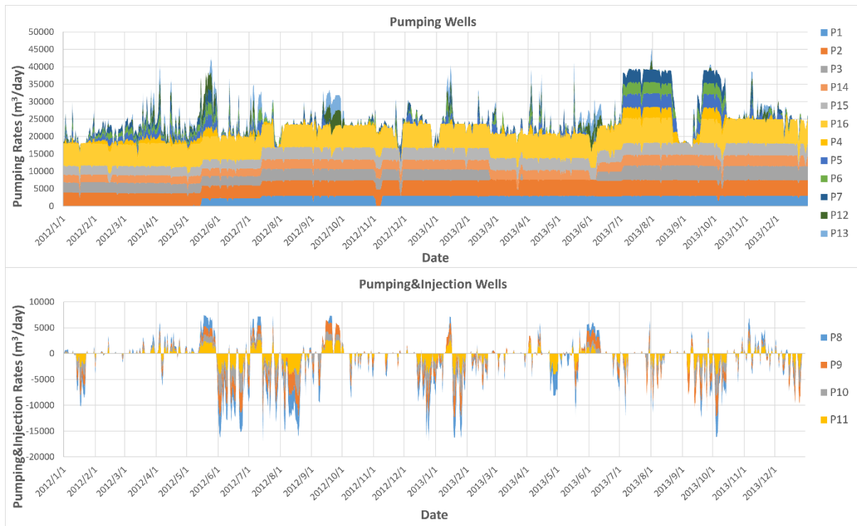
Fig. 5.3: Cumulative pumping (positive) and injection (negative) flow rates at all 16 production wells during the years of 2012 and 2013 from the WRAS+ database.
