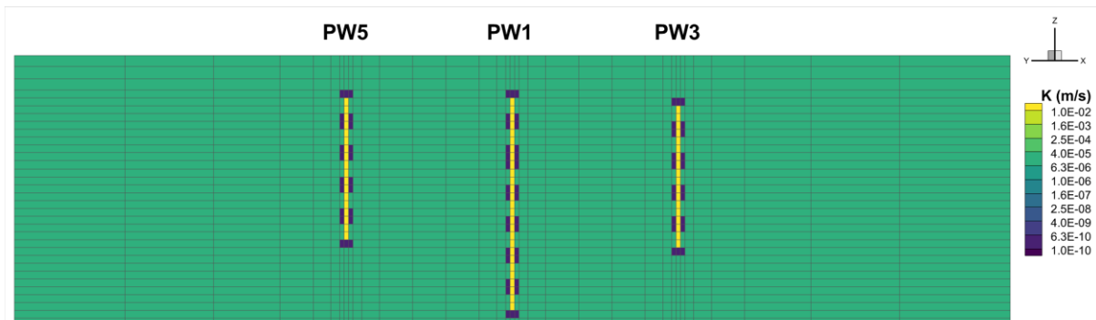
Fig. E3: Cross-section along A-B (Figure 1a) showing numerical multilevel-screened wells at the NCRS.
