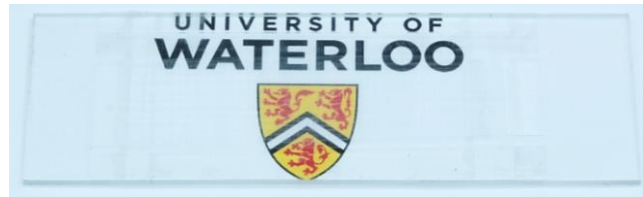
Figure 6.4. Transparency of the developed biaxially aligned porous fibers
