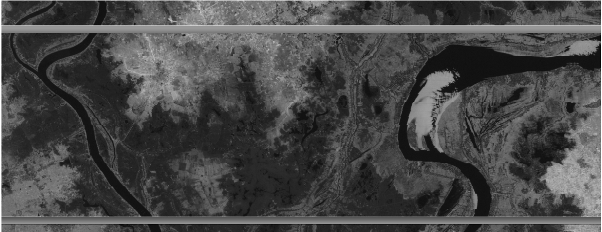
(a) Dropped Scans, Landsat 7. [71]. An entire scan line is lost due to temporary instrument or transmission issues.
