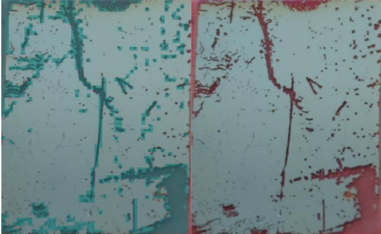
Figure 8.7: Re-trained calcium WVTR network using a red background to enhance visual contrast between degraded and intact films.
