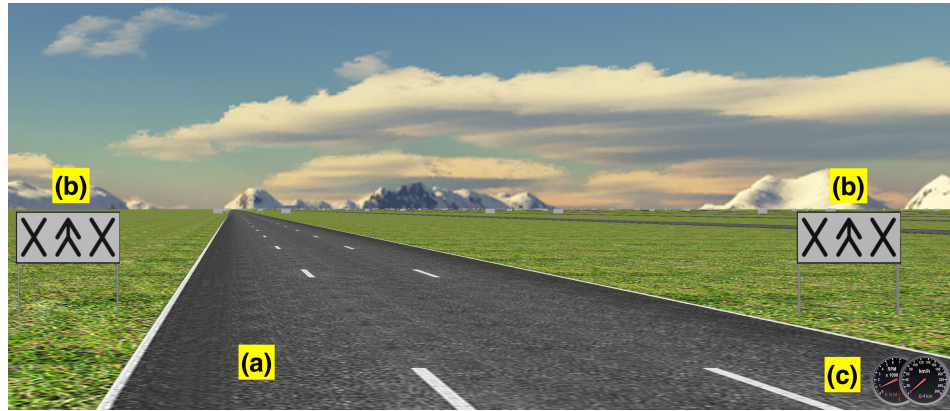
Figure 4.1: Example of lane change driving task: (a) 3-lane roadway with drive in left lane; (b) pair of signs instructing driver to change to centre lane; (c) speedometer for driver to maintain 80 km/h.
