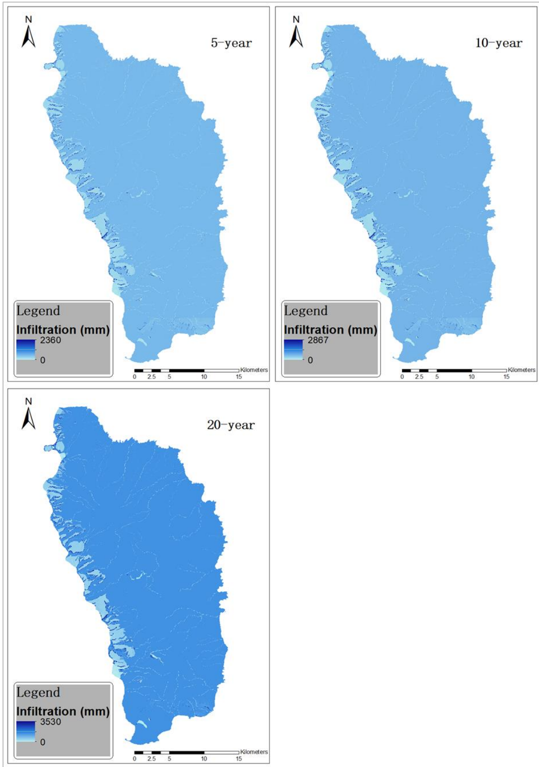
Figure B.7: Output infiltration maps for the three simulated flash flooding events. Top left: 5-year flood event; Top right: 10-year flood event; Bottom left: 20-year flood event.
