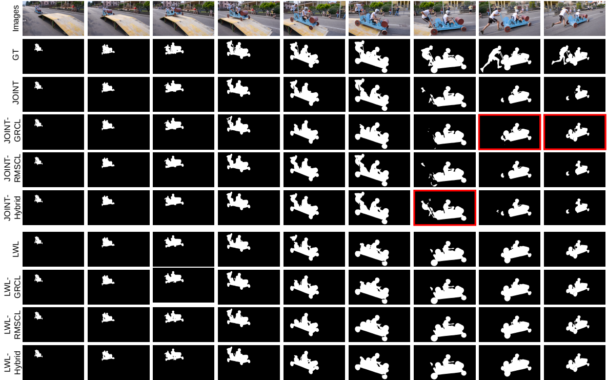
Figure 7.8: The qualitative comparison of the evaluated methods on a short video dataset (DAVIS16 [86]). The results show that the proposed GRCL, RMSCL, and Hybrid almost keep the performances of baselines intact on DAVIS16 and improve the object segmentation of some frames shown in red compared to JOINT. These qualitative results reflect the quantitative results of Table 7.2.
